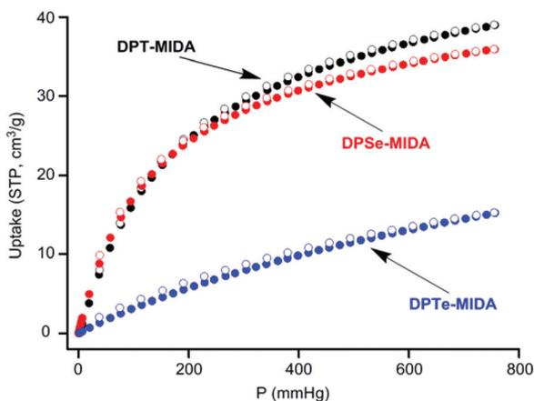
Fig. 3 CO<sub>2</sub> sorption isotherm of **DPT-MIDA**, **DPSe-MIDA** and **DPTe-MIDA** at 273 K. (filled circles: adsorption, open circles: desorption, STP = standard temperature pressure).
