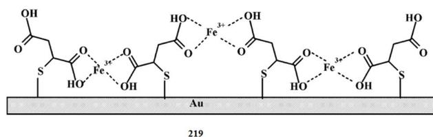
Fig. 183 Schematic for the interaction of Fe<sup>3+</sup> ions with the Au-MSA SAM electrode 219.
