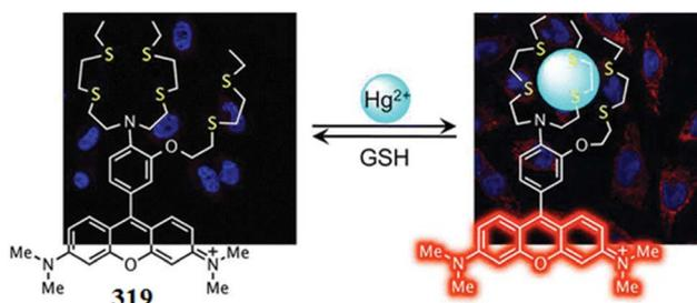
Fig. 281 Chemical structure of RosHg-based fluorescent sensor **319**, its proposed binding mode with that of  $\text{Hg}^{2+}$ , and reversibility in the presence of glutathione (GSH).
