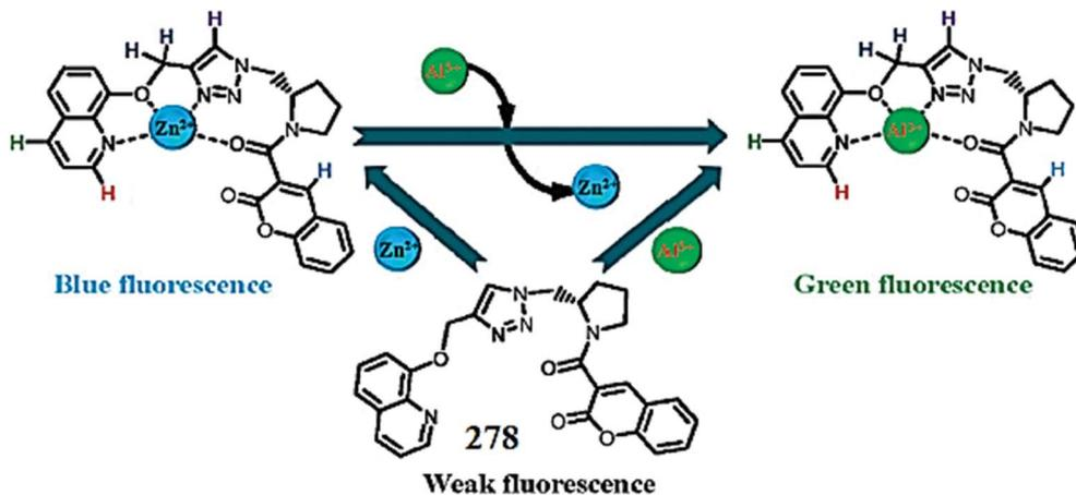
Fig. 242 Chemical structure of receptor 278 and the proposed ligand–metal complexation mechanism.
