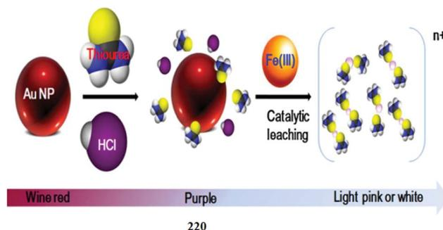
Fig. 184 Proposed mechanism for the colorimetric change of AuNPs 220 induced by Fe<sup>3+</sup> ions in the presence of an acidic thiourea system.
