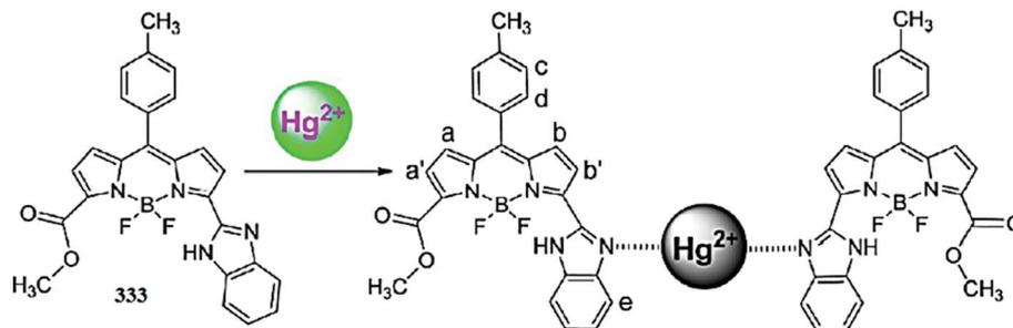
Fig. 293 Proposed binding mechanism of  $\text{Hg}^{2+}$  with ligand 333.
