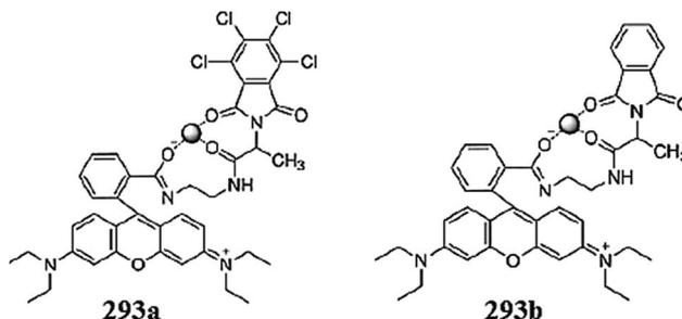
Fig. 257 Chemical structure of the ligand– $\text{Hg}^{2+}$  complexes.
