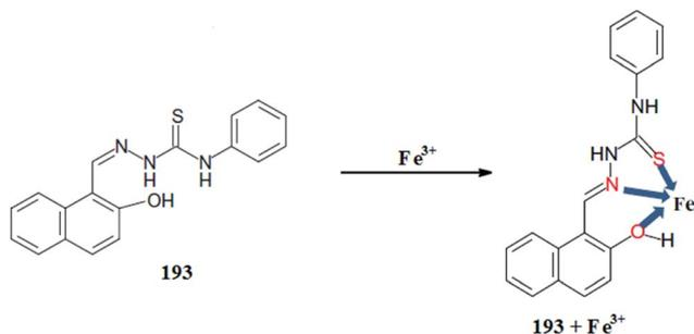
Fig. 160 Chemical structure of probe **193** and the proposed ligand-metal complexation mechanism.
