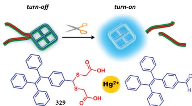
Fig. 289 Schematic of the polarity dependent chemosensor 329 for Hg<sup>2+</sup>.
