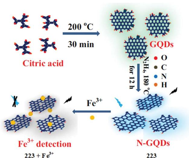
Fig. 187 Schematic of the procedure for synthesizing N-GQDs 223 and the proposed ferric ion detection mechanism.
