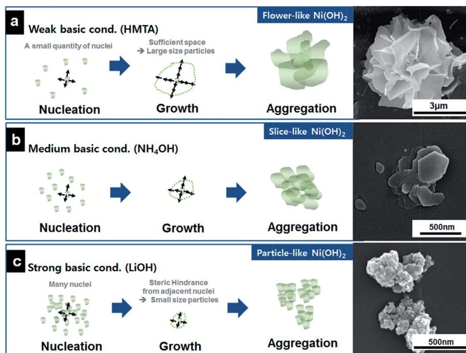
Fig. 22 Schematic diagram showing the formation process of (a) flower-, (b) slice-, and (c) particle-like  $\text{Ni(OH)}_2$  under different pH conditions; corresponding SEM Images of as-prepared samples are in the Right Panel. Reproduced with permission from ref. 244. Copyright 2013 American Chemical Society.
