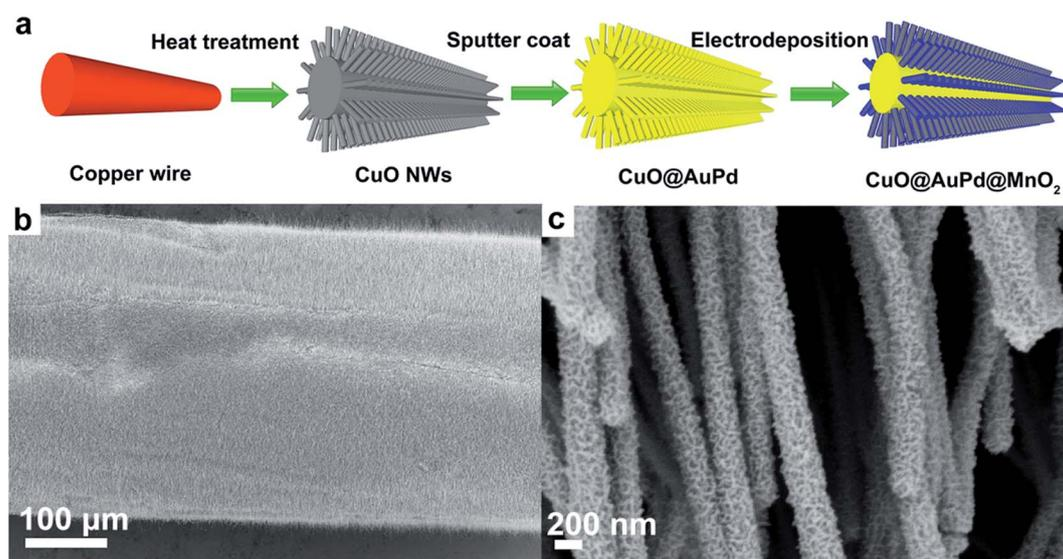
Fig. 8 (a) Schematic illustration of the fabrication process of  $\text{CuO@AuPd@MnO}_2$  NWs. (b) SEM image shows that the copper wire is completely covered by  $\text{CuO}$  NWs. (c) SEM image of  $\text{MnO}_2$  that was uniformly electrodeposited onto NWs. Reproduced with permission from ref. 83. Copyright 2014 WILEY-VCH Verlag GmbH & Co. KGaA, Weinheim.
