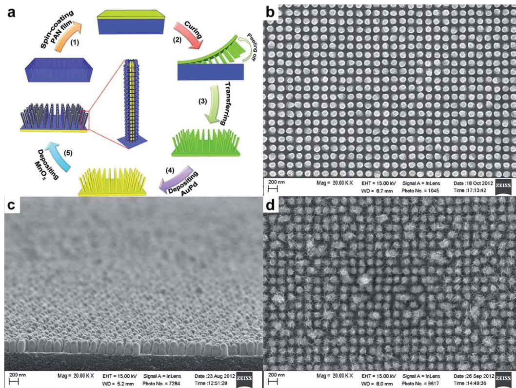
Fig. 7 (a) Schematic illustration of the development of  $\text{MnO}_2$  coated electrodes. SEM images show top (a) and side (b) view of as-printed PAN nanostructures. (d) SEM image of electrochemically deposited  $\text{MnO}_2$  nanoparticulates on pillar nanoarrays. Reproduced with permission from ref. 52. Copyright 2013 WILEY-VCH Verlag GmbH & Co. KGaA, Weinheim.
