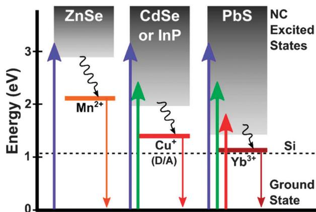
Fig. 8 Possibilities for semiconductor-dopant combinations indicating potential for covering more of the solar spectrum with for instance InP doped with  $\text{Cu}^+$ . Reproduced with permission from ref. 196.
