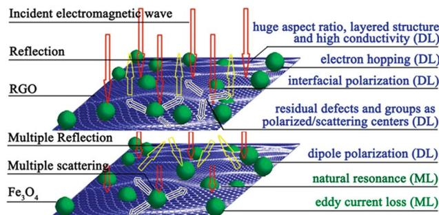
Fig. 11 Schematic of possible microwave absorbing mechanisms of the RGO-Fe<sub>3</sub>O<sub>4</sub> composites.
