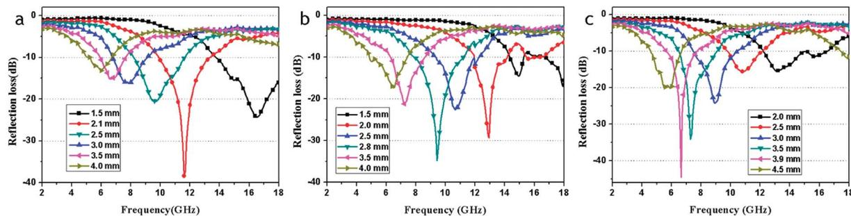
Fig. 10 The calculated reflection losses for RGO-Fe<sub>3</sub>O<sub>4</sub>-1 (a), RGO-Fe<sub>3</sub>O<sub>4</sub>-2 (b) and RGO-Fe<sub>3</sub>O<sub>4</sub>-3 (c) with different thicknesses in the frequency range of 2–18 GHz.
