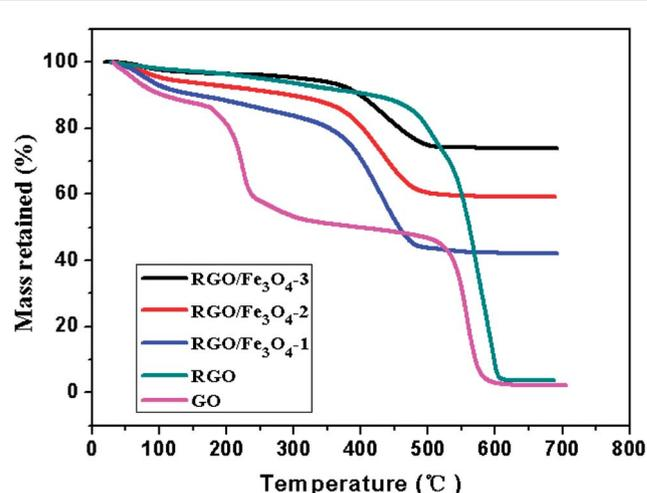
Fig. 6 TG curves of GO, RGO and RGO-Fe<sub>3</sub>O<sub>4</sub> composites in air atmosphere.
