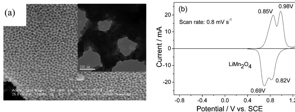
**Fig. 17** (a) SEM micrograph of the porous  $\text{LiMn}_2\text{O}_4$  and (b) CV curve of the micrometer  $\text{LiMn}_2\text{O}_4$  in the saturated  $\text{Li}_2\text{SO}_4$  solution (modified from ref. 10b and 104).
