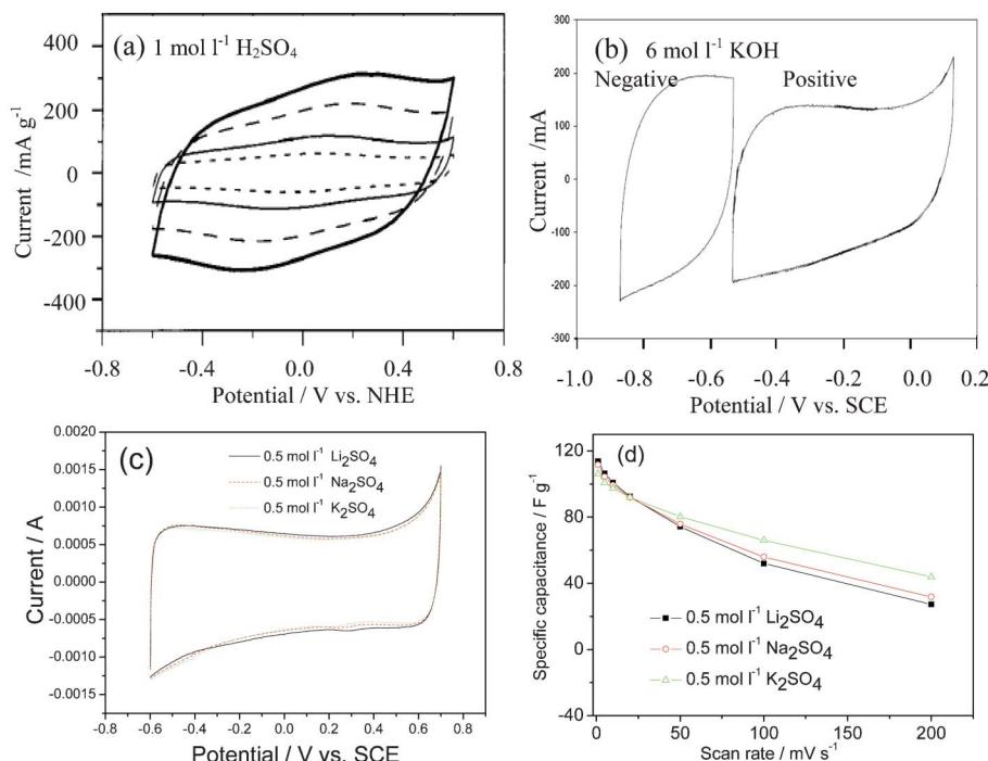
**Fig. 2** CV curves of AC as negative electrodes in different aqueous electrolytes: (a), (b) (modified from ref. 12b), (c) 0.5 mol l⁻¹ Li₂SO₄, Na₂SO₄ and K₂SO₄ solutions and (d) the change of capacitance with the scan rate in different aqueous electrolytes (modified from ref. 13). Note: Fig. 2b also shows that AC can also be positive electrodes.
