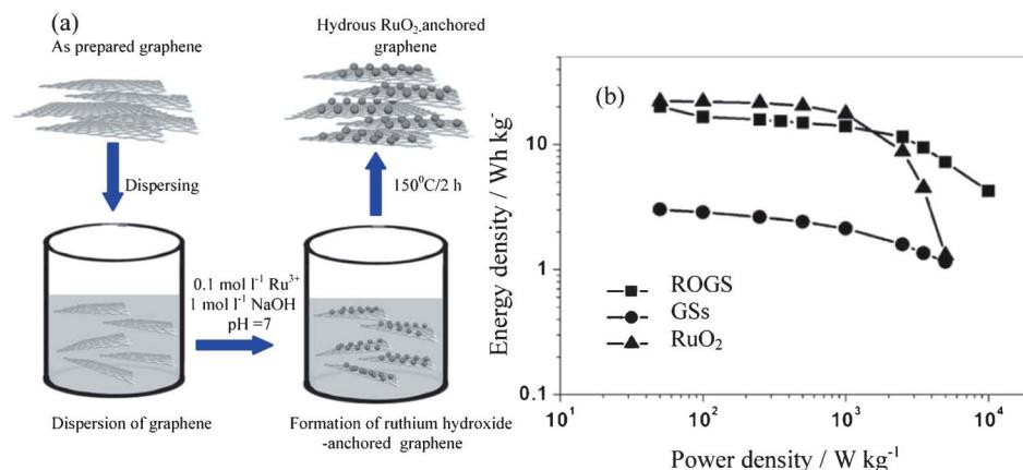
**Fig. 7** (a) The preparation scheme of RuO<sub>2</sub>/GSs composites (ROGS) and (b) Ragone plot for the as-prepared GSs, RuO<sub>2</sub>, and ROGS (Ru, 38.3 wt%) (modified from ref. 59a).
