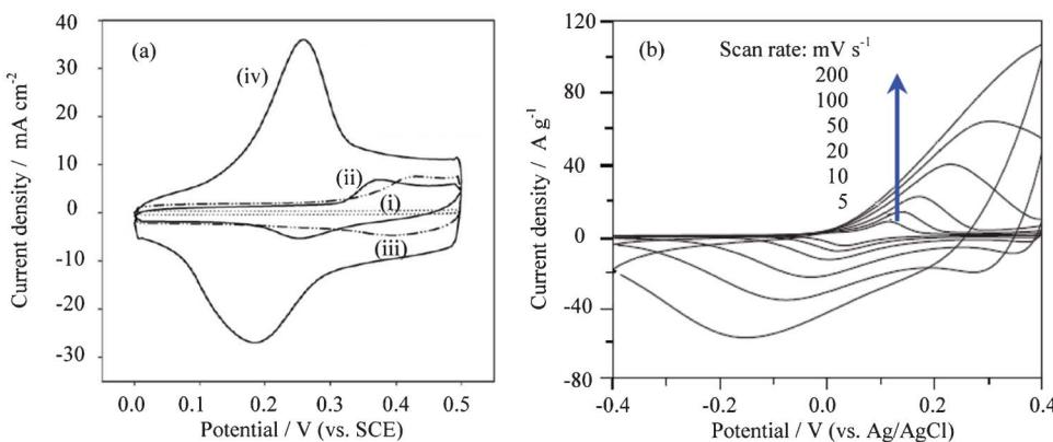
**Fig. 14** (a) CV curves of various electrodes at  $50 \text{ mV s}^{-1}$  in  $1 \text{ mol l}^{-1}$  KOH solution: (i) CNTs; (ii), nickel oxide/CNTs; (iii) cobalt oxide/CNTs; (iv), nickel-cobalt oxides/CNTs (Ni/Co molar ratio = 1 : 1), and (b) CV curves of  $\alpha\text{-Co(OH)}_2$  composite electrode recorded in  $1 \text{ mol l}^{-1}$  KOH aqueous solution at different scan rates (modified from ref. 84a and 85c).
