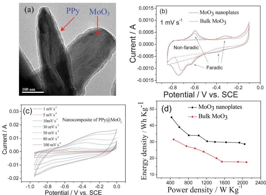
**Fig. 4** (a) TEM micrograph of PPy coated MoO<sub>3</sub> nanorods, (b) CV curves of the bulk and nanoplates MoO<sub>3</sub>, (c) CV curves of the PPy@MoO<sub>3</sub> nanocomposite at different scan rate and (d) Ragone plot of the ASCs based on MoO<sub>3</sub>//AC in 0.5 mol l<sup>-1</sup> Li<sub>2</sub>SO<sub>4</sub> solution (modified from ref. 6c and 49c).
