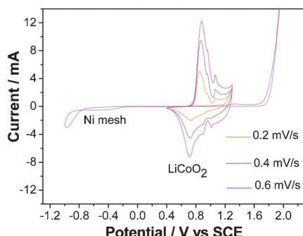
**Fig. 16** CV curves of  $\text{LiCoO}_2$  and nickel mesh in saturated  $\text{Li}_2\text{SO}_4$  solution (modified from ref. 92).
