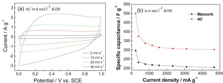
**Fig. 6** (a) CV curves of an AC in  $6 \text{ mol l}^{-1}$  KOH aqueous electrolyte and (b) comparison of gravimetric capacitances against current density for the AC and the commercial Maxsorb carbon (modified from ref. 51b).
