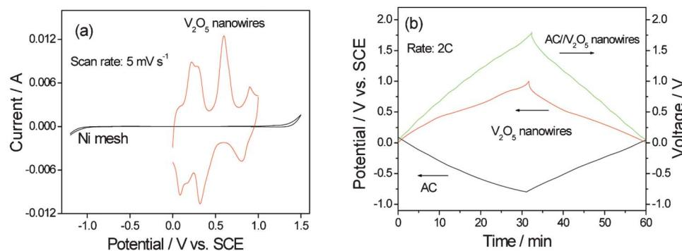
**Fig. 12** (a) CV curve of  $\text{V}_2\text{O}_5$  nanowires and Ni mesh (current collector) and (b) charge/discharge curves of AC// $\text{V}_2\text{O}_5$  nanowires in 0.5 mol l<sup>-1</sup> K<sub>2</sub>SO<sub>4</sub> aqueous solution (modified from ref. 6a).
