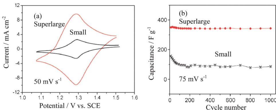
**Fig. 13** (a) Typical CV curves and (b) cycling performance of super-large  $\text{PbO}_2$  dendrites composed of trigonal nanoplates and the small dendrites in  $5.0 \text{ mol l}^{-1} \text{H}_2\text{SO}_4$  solution recorded a scan rate of  $75 \text{ mV s}^{-1}$  (modified from ref. 82c).
