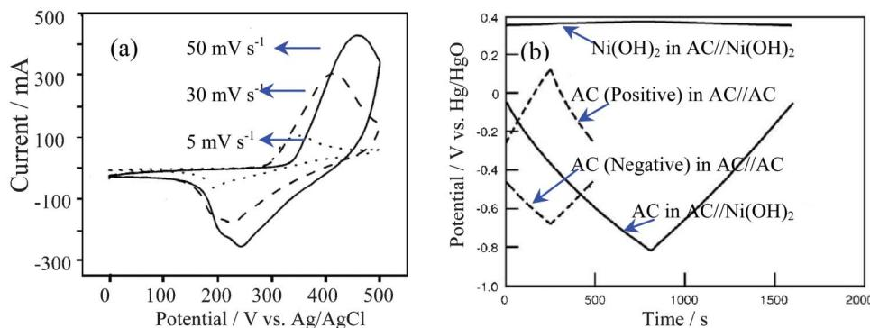
**Fig. 15** (a) CV curve of  $\text{Ni(OH)}_2$  in alkaline solution and (b) charge/discharge curves of the positive and negative electrodes in the  $\text{AC//Ni(OH)}_2$  ASC and electric double layer capacitors of  $\text{AC//AC}$  at  $1 \text{ mA cm}^{-2}$  in  $10 \text{ mol l}^{-1}$  KOH aqueous solution (modified from ref. 87b and 90c).
