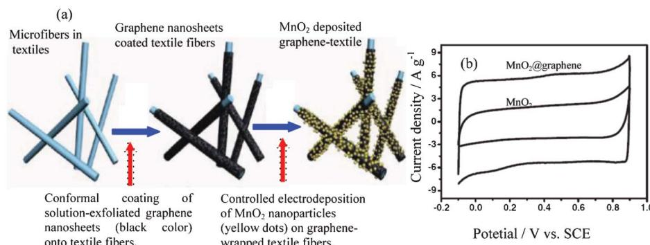
**Fig. 9** (a) Schematic illustration of two key steps for preparing hybrid MnO<sub>2</sub>-nanostructured textiles@graphene and (b) CV curves of an optimized MnO<sub>2</sub>@graphene at different potential windows at the scan rate of 20 mV s<sup>-1</sup> in 1 mol l<sup>-1</sup> Na<sub>2</sub>SO<sub>4</sub> solution (modified from ref. 8a and 8b, respectively).
