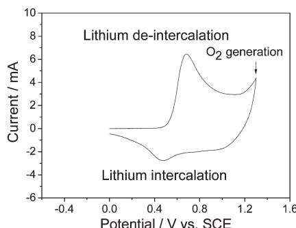
**Fig. 18** CV curve of  $\text{LiNi}_{1/3}\text{Co}_{1/3}\text{Mn}_{1/3}\text{O}_2$  in  $2 \text{ mol l}^{-1}$   $\text{Li}_2\text{SO}_4$  aqueous solution (modified from ref. 108).
