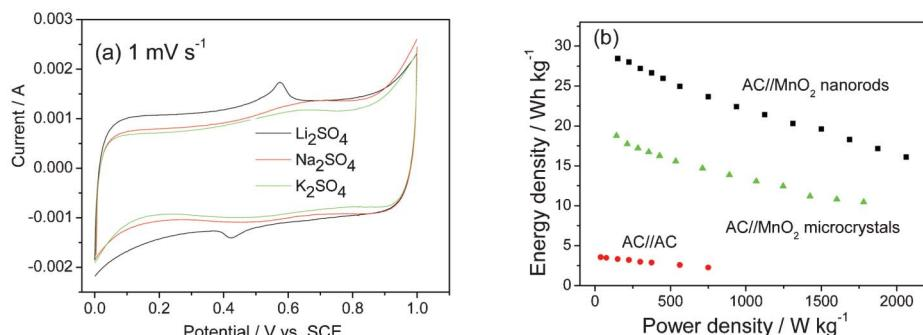
**Fig. 10** (a) CV curve of MnO<sub>2</sub> in 0.5 mol l<sup>-1</sup> different neutral electrolytes and (b) Ragone plots of the hybrid supercapacitors AC//MnO<sub>2</sub> nanorods, AC//MnO<sub>2</sub> microcrystals supercapacitor and AC//AC supercapacitor in 0.5 mol l<sup>-1</sup> K<sub>2</sub>SO<sub>4</sub> electrolyte (modified from ref. 7c).
