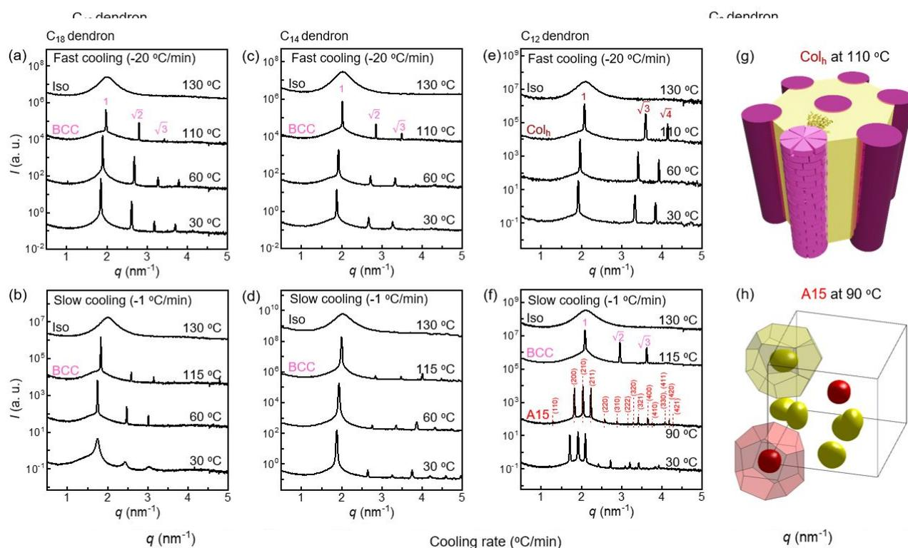
**Fig. 2** SAXS intensity profiles of (a,b)  $C_{18}$ , (c,d)  $C_{14}$ , and (e,f)  $C_{12}$  dendrons with two different cooling rates of  $-20$  and  $-1$   $^{\circ}\text{C}/\text{min}$  from  $130$  to  $30$   $^{\circ}\text{C}$ . 3D morphologies reproduced from the ED maps of (g) the stacked  $\text{Col}_h$  and (h) A15 phases, which are obtained from the fast and slow cooling of the  $C_{12}$  dendrons, respectively.
