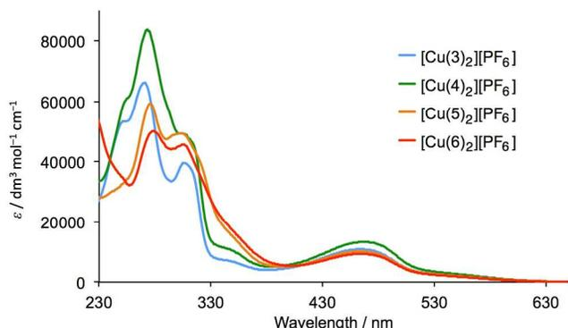
Fig. 2. Solution ( $\text{CH}_2\text{Cl}_2$ ) absorption spectra of complexes  $[\text{Cu}(\text{L}_{\text{ancillary}})_2][\text{PF}_6]$  with  $\text{L}_{\text{ancillary}} = \mathbf{3-6}$  ( $5 \times 10^{-5} \text{ mol dm}^{-3}$ ).
