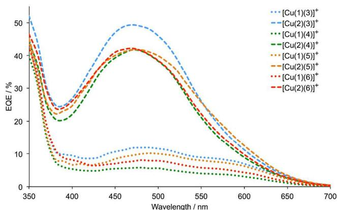
**Fig. 7.** EQE spectra for DSCs containing the dyes  $[\text{Cu}(1)(\text{L}_{\text{ancillary}})]^+$  and  $[\text{Cu}(2)(\text{L}_{\text{ancillary}})]^+$  ( $\text{L}_{\text{ancillary}} = 3-6$ ) measured on the day the DSCs were made.
