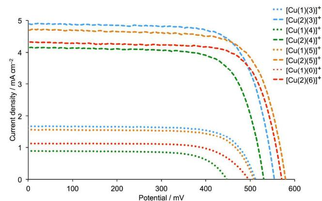
Fig. 6.  $J-V$  curves for DSCs containing the dyes  $[\text{Cu}(\mathbf{1})(\text{L}_{\text{ancillary}})]^+$  and  $[\text{Cu}(\mathbf{2})(\text{L}_{\text{ancillary}})]^+$  ( $\text{L}_{\text{ancillary}} = \mathbf{3-6}$ ) measured on the day the DSCs were assembled.
