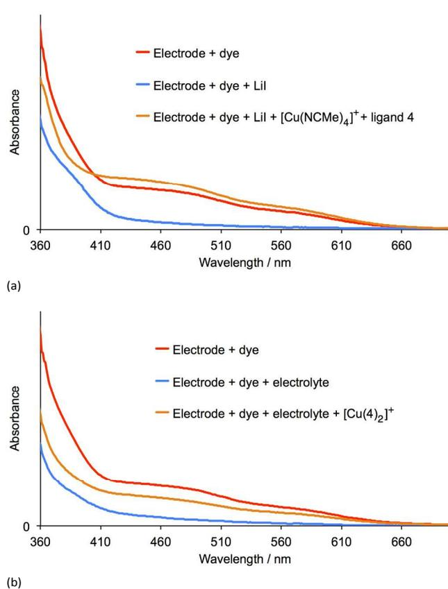
Fig. 9. Solid-state absorption spectra of transparent electrodes (no scattering layer on the  $\text{TiO}_2$ ) functionalized with the dye  $[\text{Cu}(\mathbf{1})(\mathbf{4})]^+$  (red) and post-treated (a) with Lil solution (blue), then  $[\text{Cu}(\text{NCMe})_4][\text{PF}_6]$  followed by ligand  $\mathbf{4}$  (orange), and (b) with  $\text{I}^-/\text{I}_3^-$  electrolyte (blue), then  $[\text{Cu}(\mathbf{4})_2]^+$ .
