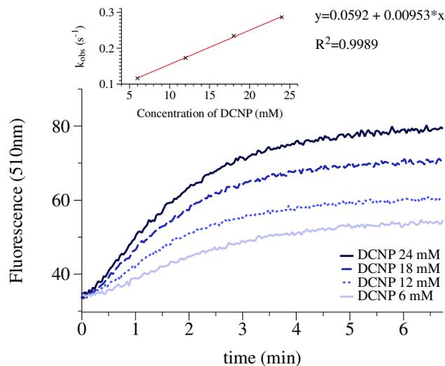
Figure 3. Kinetic profile of the emission intensity at 510 nm of probe **2** after the addition of 6, 12, 18 and 24 mM DCNP. Probe **2** is  $10^{-6}$  M in pH=5.5 buffered water/acetonitrile 3:1 v/v mixture. The inset shows the correlation between  $k_{\text{obs}}$  and concentration of DCNP.
