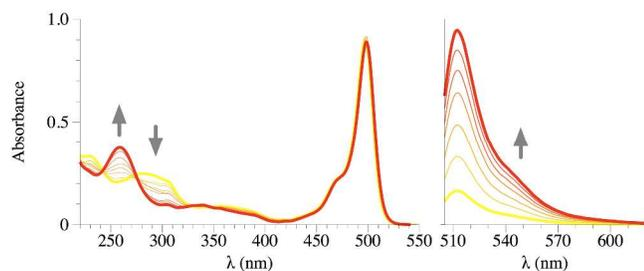
Figure 2. UV-vis (left) and emission (right,  $\lambda_{\text{exc}}=470$  nm) spectra of compound **2** in MeCN ( $1 \times 10^{-6}$  M for emission,  $1 \times 10^{-5}$  M for UV-vis) titrated with DCNP (from 100  $\mu\text{M}$  to 20 mM). Yellow: free ligand, red: ligand+DCNP 20 mM
