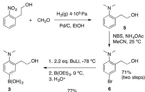
Scheme 4. Synthetic procedures to form the boronic acid of sensing unit **3**.
