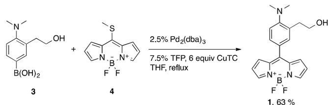
Scheme 3. Coupling reaction to form probe **1**
