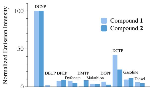
Figure 4. Relative (to DCNP) emission intensity of compounds **1** and **2** (measured at 520 and 510 nm respectively) with 1000 ppm<sub>v</sub> of DCNP, OP compounds, gasoline and diesel.
