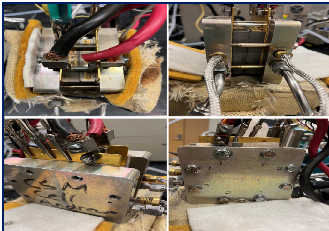
Fig. 3 Photographs of the top view and side view of a real-time fuel cell.
