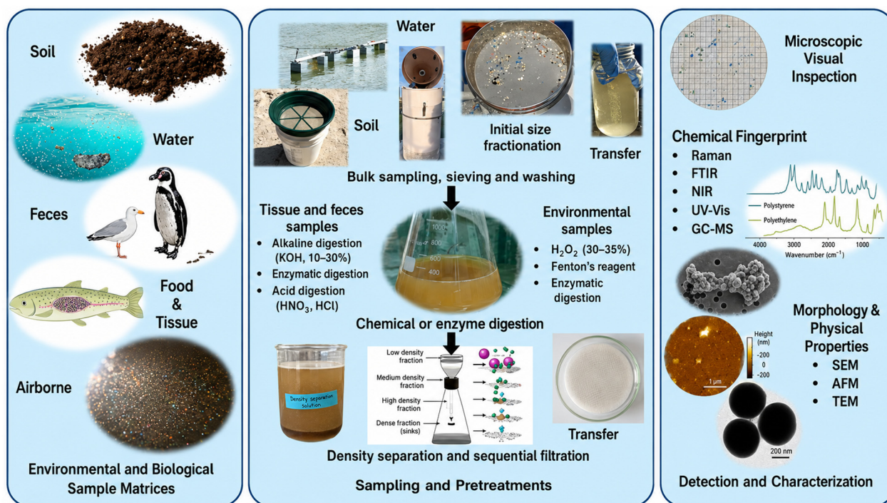
Fig. 1 Conventional workflow of MPs/NPs sampling, detection, and characterization. In general, initial sampling step relies on bulk sampling, followed by size-based fractionation and collection into glass container transferred back to laboratory for further processing. Then, different types of samples utilize different digestion reagents followed by density based separation, the supernatant goes through sequential filtration and isolate particles of interests of variety of sizes, finally trapped on membrane filters for characterizations. Depends on the nature of downstream characterization techniques, further processing of the filter paper is required.
