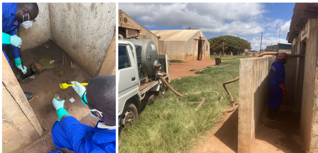
Fig. 2 Sample collection, Dzaleka camp. (A) Pit latrine grab sample collection. (B) Pump truck sample collection.
