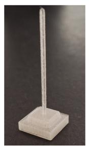
Fig. 1 Temperature sensor fabricated using fluorindate glass through 3D
