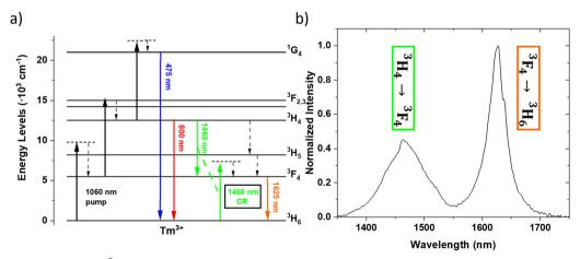
Fig. 2 (a) Energy level diagram of Tm<sup>3+</sup> illustrating the photon-avalanche process under 1060 nm excitation. (b) Near-infrared emission spectrum of studied material under 1060 nm excitation.
