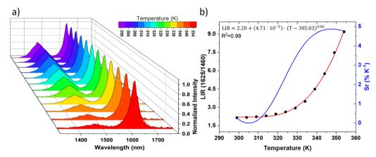
Fig. 4 (a) Emission spectrum in the IR range under 1060 nm excitation. (b) LIR and relative sensitivity as a function of temperature.
