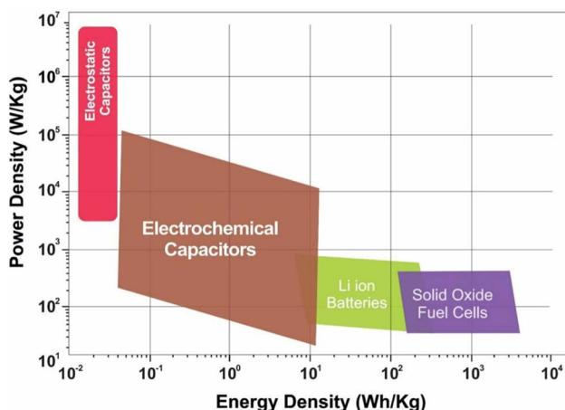
Fig. 1 Ragone plot comparing various energy storage systems. Reproduced with permission<sup>5</sup> copyright 2018, Elsevier.
