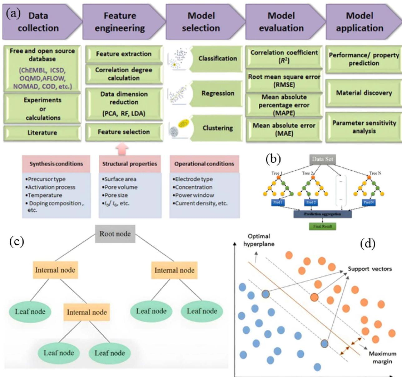
**Fig. 11** (a) Systematic framework for predicting supercapacitor performance using ML. Reproduced with permission.<sup>134</sup> Copyright 2024, Elsevier. (b) Schematic of random forest. Reproduced with permission.<sup>130</sup> Copyright 2025, Elsevier. (c) Schematic representation of decision tree. Reproduced with permission.<sup>130</sup> Copyright 2025, Elsevier. (d) Schematic representation of SVM. Reproduced with permission.<sup>130</sup> Copyright 2025, Elsevier.
