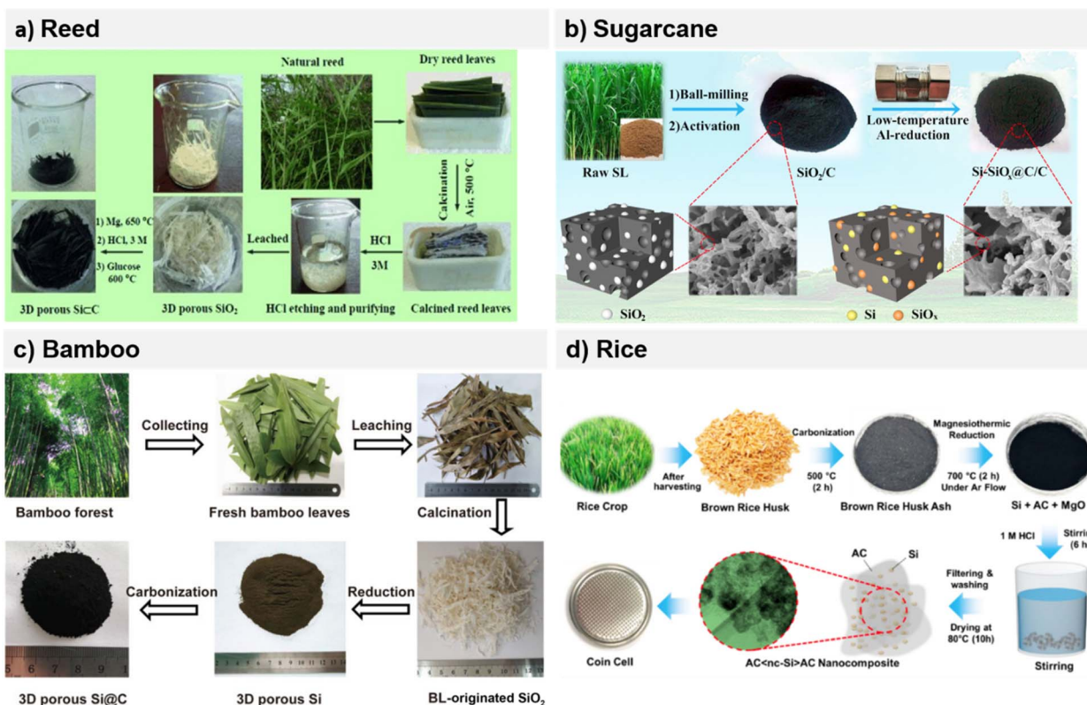
Fig. 1 Representative processes reported for the utilization of siliceous plants as bioprecursors for Si-based anodes: (a) reed plant, reproduced from ref. 36 with permission, copyright [2015], (b) sugarcane, reproduced from ref. 69, copyright © 2021, (c) bamboo, reproduced from ref. 75, copyright © 2022, and (d) rice, reproduced from ref. 80, copyright © 2019.
