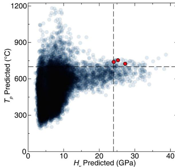
**Fig. 5** Predicted Vickers microhardness ( $H_V$ ) plotted against predicted oxidation temperature ( $T_p$ ) for 15 247 pseudo-binary and ternary inorganic compounds extracted from the Materials Project. Dashed lines at 24 GPa and 700 °C represent thresholds for hardness and thermal stability, respectively. Three target compounds selected for future experimental validation are highlighted in red.
