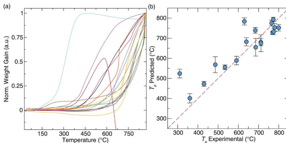
Fig. 4 (a) Thermogravimetric analysis curves for the validation dataset, measured in air up to 870 °C, showing normalized weight gain profiles. (b) Correlation of experimental  $T_p$  oxidation temperature with predictions for the optimized machine learning model. The dashed red line denotes a 1:1 correlation. Error bars indicate the standard deviation across bagged estimators.
