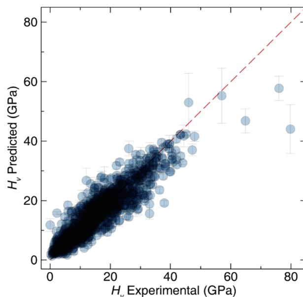
Fig. 2 Experimentally measured Vickers microhardness ( $H_{V,\text{exp}}$ ) plotted against the predicted values ( $H_{V,\text{pred}}$ ) from the XGBoost model for 1225 inorganic compounds. Error bars represent the standard deviation across three bagging estimators. The red dashed line indicates the ideal fit.
