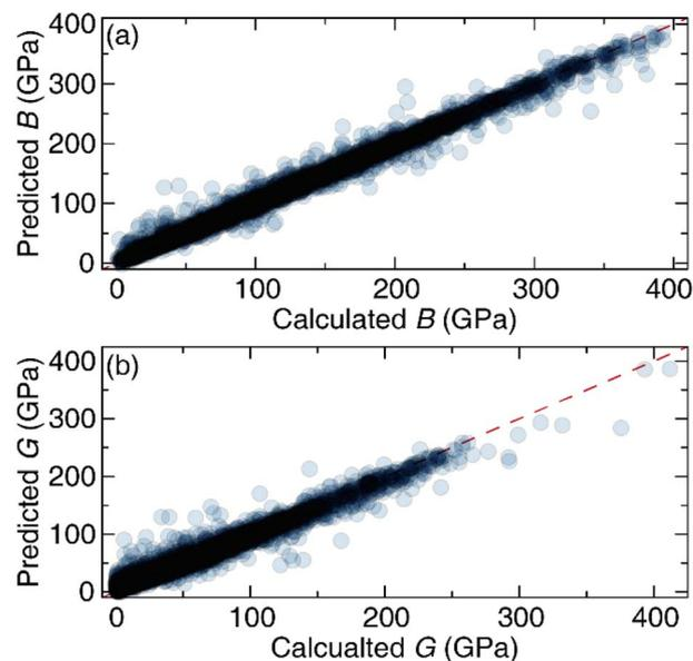
Fig. 1 Predicted versus DFT-calculated elastic moduli for the (a) bulk modulus ( $B$ ) and (b) shear modulus ( $G$ ) using the extreme gradient boosting model trained on 7148 inorganic compounds. DFT-calculated values were obtained from the Materials Project database. Model performance was evaluated using 10-fold cross-validation. The red dashed line represents the ideal 1 : 1 parity line.
