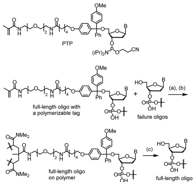
**Scheme 1** Catching-by-polymerization (CBP). Conditions: (a) *N,N*-dimethylacrylamide, *N,N'*-methylenebis(acrylamide), sodium acrylate, ammonium persulfate, *N,N,N',N'*-tetramethylethylenediamine (TMEDA), rt, 1 h. (b) Wash. (c) AcOH (80%), rt, 5 min  $\times$  3. PTP = polymerizable tagging phosphoramidite. B = nucleobase.
