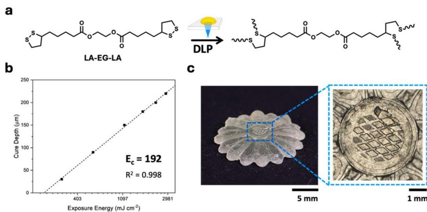
**Fig. 2** (a) Photopolymerisation reaction of LA-EG-LA for the formation of a polymer network during the DLP printing process. (b) Jacobs working curves of LA-EG-LA with an LED at 405 nm. (c) 3D printed flower printed with a layer thickness of 100  $\mu\text{m}$  and a light intensity of 55  $\text{mW cm}^{-2}$ , light microscope image showing the highly detailed centre of the 3D printed flower.
