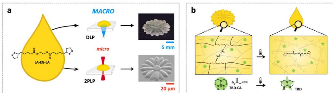
**Fig. 1** (a) 3D printing process on the macro- and micro-scale: a difunctional crosslinker (LA-EG-LA) synthesised from bio-based starting materials – lipoic acid and ethylene glycol – is used without the need of additional additives for 3D printing using digital light processing (DLP) and two-photon laser printing (2PLP). (b) Latent base activated depolymerisation of 3D printed structures is performed by thermal activation, enabling controlled depolymerisation across both printing scales.
