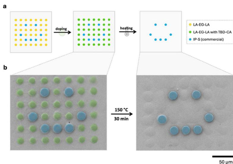
**Fig. 6** (a) Schematic representation of the multi-material printing process and the subsequent doping and depolymerisation of the 3D microprinted structures, (b) SEM images of an array of pillars printed with IP-S and LA-EG-LA before and after heating to 150 °C, causing the pillars of LA-EG-LA doped with TBD-CA to depolymerise (subsequently coloured for visual distinction).
