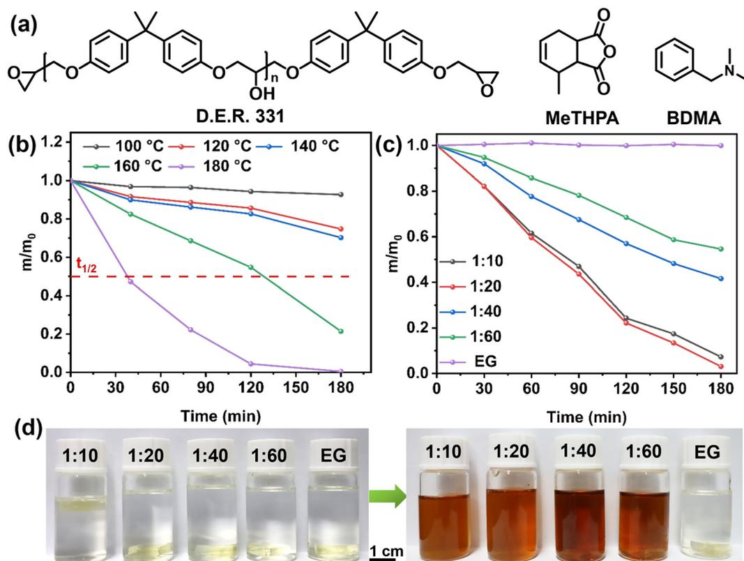
Fig. 3 (a) Molecular formulae for epoxy degradation formulations; normalized mass vs. time for epoxy degradation at different temperatures (b) and varying DES concentrations (c); and (d) photographs of the solutions before and after degradation.
