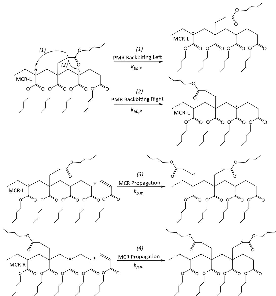
**Fig. 4** Top: Two backbiting reactions for PMR, for simplicity L(left) and R(right); Bottom: follow-up propagations.
