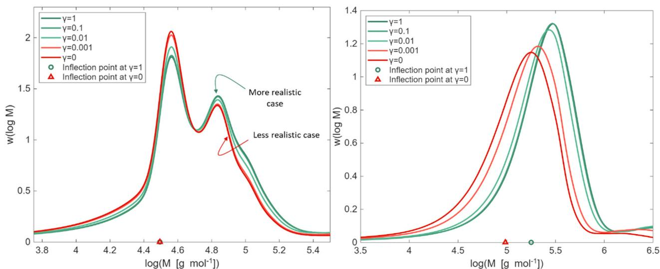
**Fig. 5** Left: kMC simulation of bulk PLP of *n*BuA at a laser pulse frequency of 500 Hz and 306 K, with a variation of  $\gamma$  (eqn (2);  $\gamma = 1$  implying  $k_{p,p} = k_{p,e}$  and  $\gamma = 0$  implying  $k_{p,p} = k_{p,m}$ ). Right similar plot but at a lower laser pulse frequency of 50 Hz; on the x-axis the identification of the first inflection points (left coinciding; right shift). Same coloring as in Fig. 3, regarding expected behavior.
