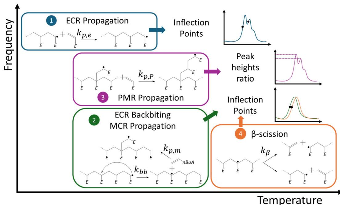
**Fig. 8** Roadmap to determine acrylate specific intrinsic rate coefficients, using PLP technique in combination with kMC simulations; not shown is the determination of  $k_{bb,P}$  for which branching densities can be used in Step 3, although likely  $k_{bb,P}$  is seen as  $k_{bb}$ .
