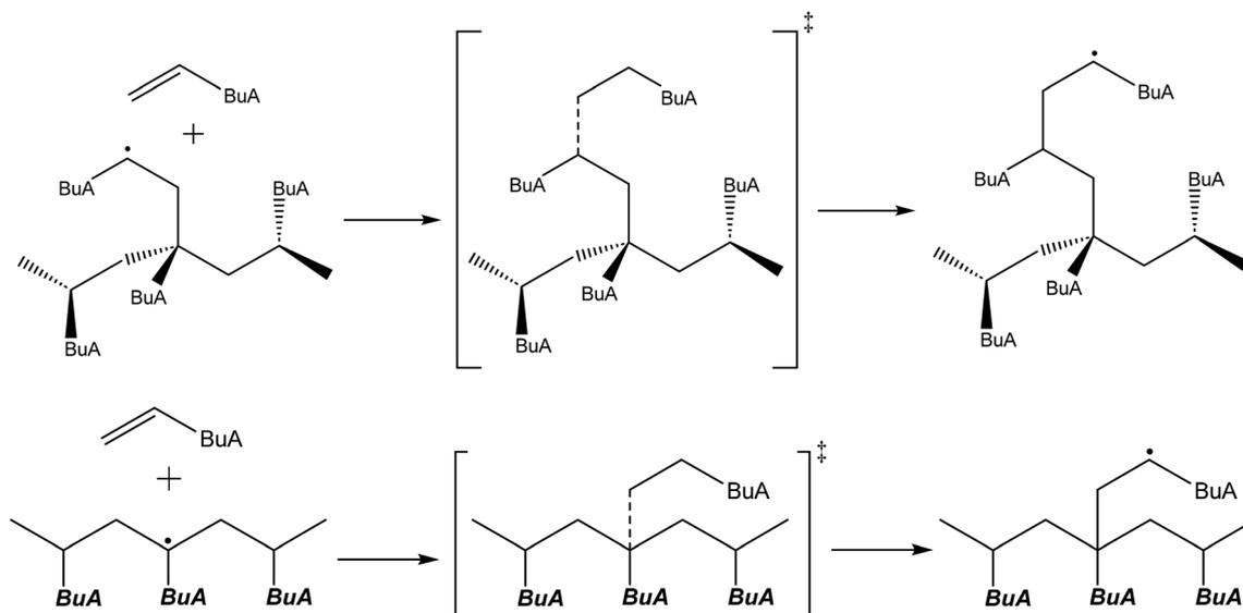
**Fig. 2** Top: Molecular model used to predict the propagation rate coefficient of the propagated mid-chain radical (PMR). It consists of a tetramer radical, propagating towards a monomer. Bottom: Molecular model used to predict the propagation rate coefficient of the mid-chain radical (MCR). It consists of a trimer radical, propagating towards a monomer.
