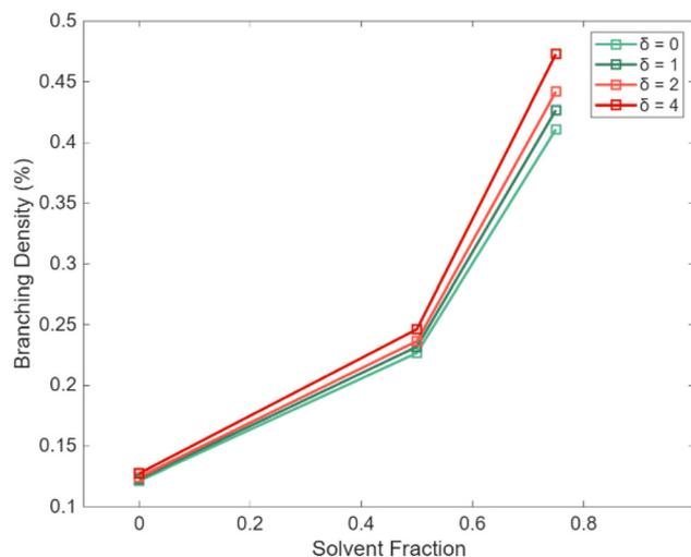
**Fig. 7** Branching density as a function of the solvent fraction for different  $\delta$  (eqn (3)) values; PLP conditions: 500 Hz, at 306 K, fixing the value of  $\gamma$  to 1. In practice, one likely will end up setting  $\delta$  equal to 1.
