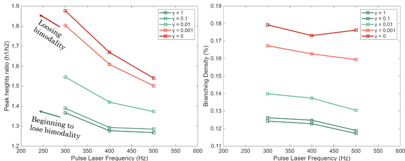
**Fig. 6** Left peak heights ratio at different values of  $\gamma$  (eqn (2)) for PLP of *n*BuA at a laser pulse frequency of 500 Hz, at 306 K, and in bulk. The green lines represent the more likely values of  $\gamma$  within the 1–0.01 range (see Fig. 1), and the red lines represent the more unlikely values of  $\gamma$  between 0.001–0. Right Corresponding branching densities.
