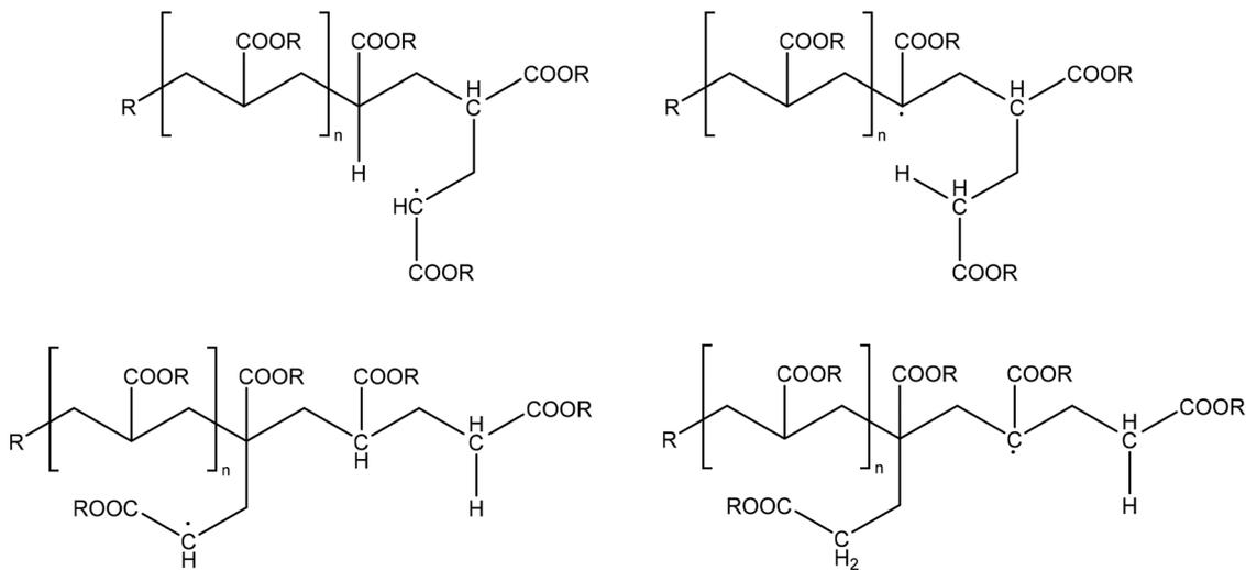
**Fig. 1** Top: End-chain radical (ECR) for acrylate radical polymerization (left); mid-chain radical (MCR) formed through backbiting over a six-membered transition state out of this ECR (right). Bottom: (left) Extra species explored in the present work, being a propagated mid-chain radical (PMR) as well (right) a new MCR after backbiting of this PMR.
