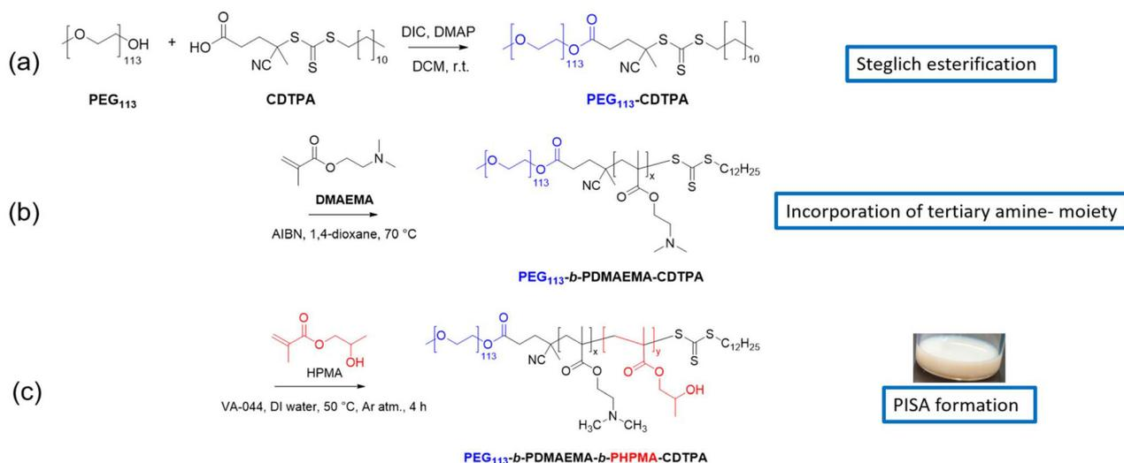
**Scheme 1** (a) Synthesis of  $\text{PEG}_{113}\text{-CDTPA}$  via Steglich esterification. (b) Synthesis of  $\text{PEG}_{113}\text{-}b\text{-PDMAEMA-CDTPA}$  to incorporate the tertiary amine moiety responsible for anchoring MNPs. (c) Synthesis of  $\text{PEG}_{113}\text{-}b\text{-PDMAEMA-}b\text{-PHPMA-CDTPA}$  triblock copolymers via thermal RAFT-PISA to form milky stable suspensions.
