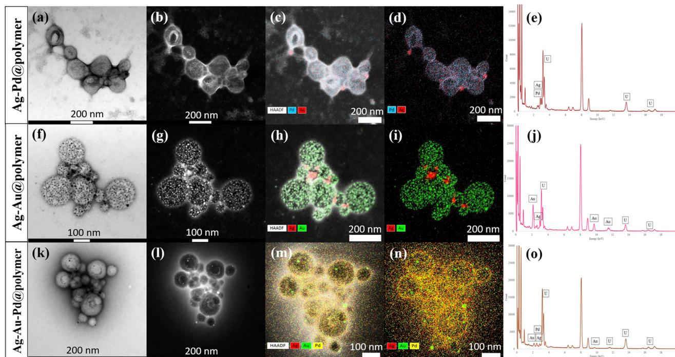
**Fig. 3** STEM images of Ag-Pd, Ag-Au and Ag-Au-Pd@PEG<sub>113</sub>-*b*-PDMAEMA<sub>32</sub>-*b*-PHPMA<sub>398</sub>-CDTPA PMNCs in (a), (f) and (k) bright-field and (b), (g) and (l) HAADF modes. (c), (h) and (m) Overlapped bright-field and STEM-EDX mapping. (d), (i) and (n) STEM-EDX-mapping. (e), (j) and (o) EDX elemental analysis.
