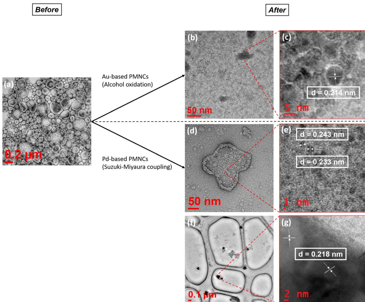
Fig. 4 TEM images of (a) Au@PEG<sub>113</sub>-PDMAEMA<sub>32</sub>-PHPMA<sub>400</sub> PMNC before subjecting to organic reactions. After subjecting to catalytic treatment: (b) Magnified view of a MNP cluster with (c) MNP inset d-spacing of 0.214 nm. (d) Amorphous-like particles with (e) MNP inset d-spacing of 0.233 nm and 0.243 nm. (f) Unusual shapes of MNPs with (g) inset d-spacing of 0.218 nm indicating possible Ag–Pd–Au alloy formations.
