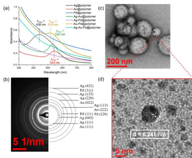
**Fig. 2** (a) UV-vis spectra of different combinations of Au/Ag/Pd@PEG<sub>113</sub>-*b*-PDMAEMA<sub>32</sub>-*b*-PHPMA<sub>398</sub>-CDTPA PMNCs. (b) SAED patterns of Ag-Au-Pd@PEG<sub>113</sub>-*b*-PDMAEMA<sub>32</sub>-*b*-PHPMA<sub>398</sub>-CDTPA. (c) TEM image of the same PMNC. (d) High-resolution TEM (HR-TEM) image of an Ag-Au-Pd metal nanoparticle (with an inset interplanar distance, *d*).
