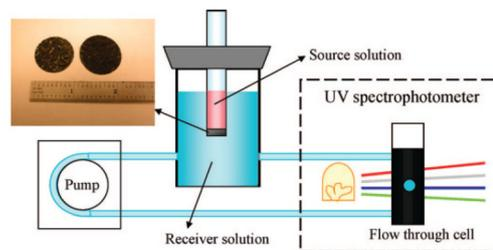
Fig. 16 Schematic setup used by Hou et al.<sup>176</sup> Reproduced from ref. 176 with permission from ACS, copyright 2025.
