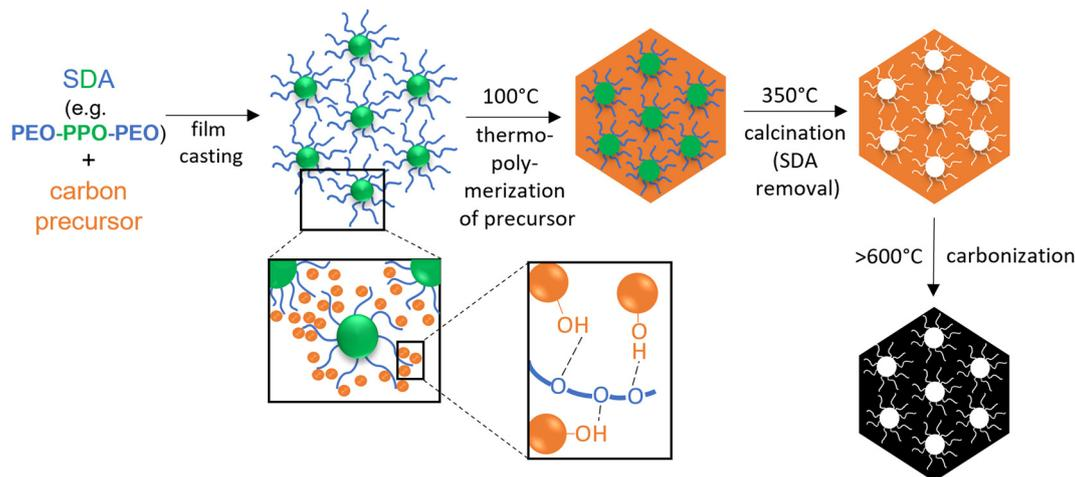
**Fig. 2** Scheme of SDA/carbon precursor self-assembly through the soft-templating process, according to Dai.<sup>45</sup>
