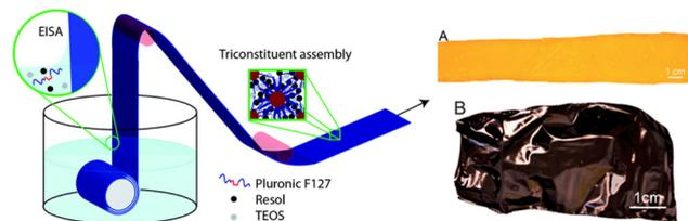
**Fig. 6** Left: Schematic synthesis of OMC films on plastic substrate. The *Kapton* substrate is submerged in a solution containing TEOS (silica source), resol (carbon precursor) and Pluronic F127 (template). Drawing the *Kapton* through the surface of the solution deposits a nanostructured coating through EISA. Right: *Kapton* after dip coating (A) and after carbonization (B). Reproduced from ref. 24 with permission from ACS, copyright 2025.
