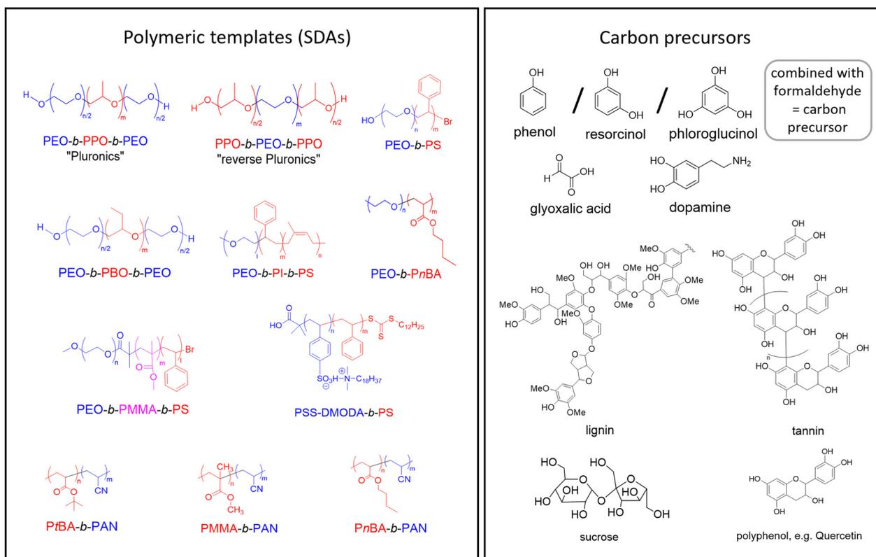
**Fig. 1** Left: SDAs that have been employed for OMC preparation *via* soft-templating. Red = lipophilic, blue = hydrophilic moieties. PEO: poly(ethylene oxide), PPO: poly(propylene oxide), PS: polystyrene, PEA: poly(ethylene adipate), PSS-DMODA: poly(*N,N*-dimethyl-*n*-octadecylammonium *p*-styrenesulfonate), PBA: poly(*n*-butyl acrylate), PtBA: poly(*tert*-butyl acrylate), PAN: polyacrylonitrile, PMMA: poly(methyl methacrylate), PI: polyisoprene. Right: Frequently applied carbon precursors.
