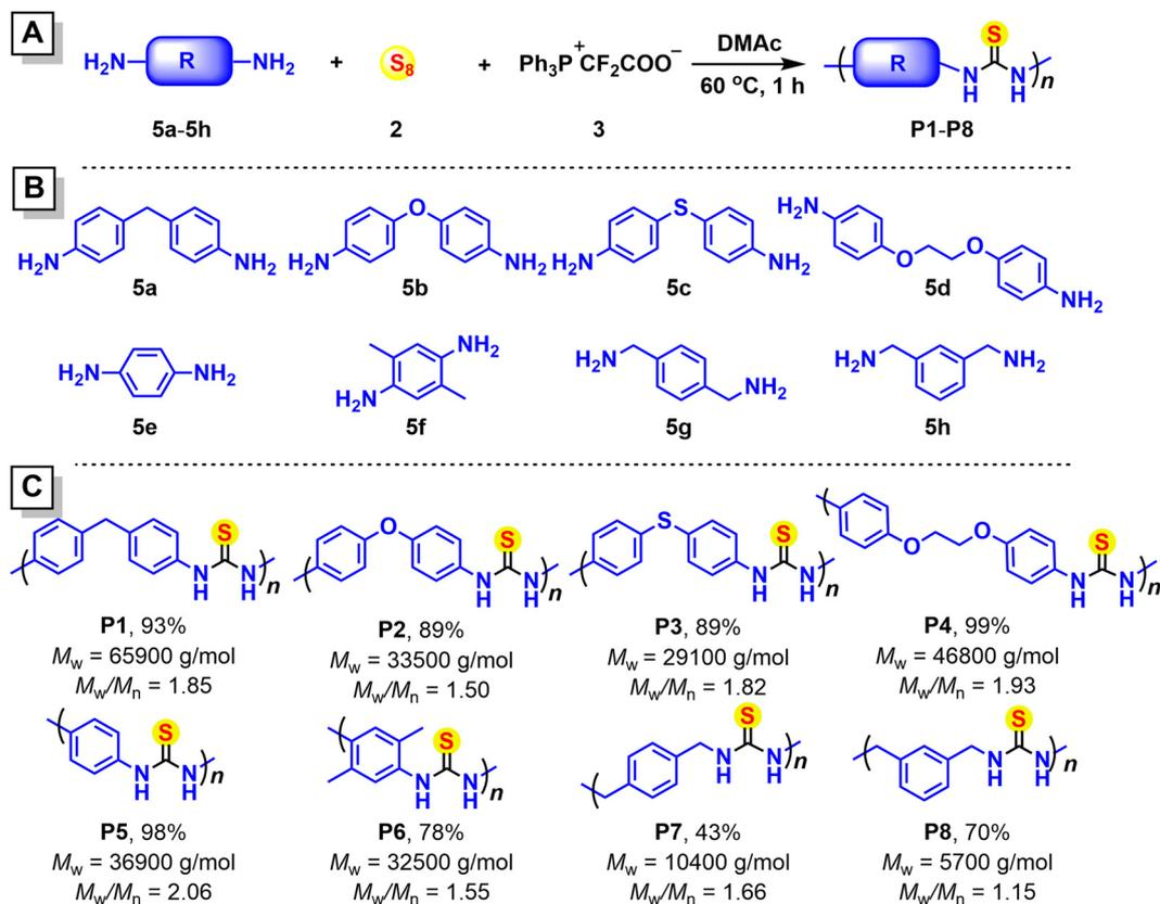
**Fig. 4** (A) The MCPs of elemental sulfur, PDFSA and diamine monomers, (B) the structures of the electron-donating-group-containing aromatic diamines 5a–5h, and (C) the chemical structures and polymerization results for P1–P8.  $M_w$ s are determined using GPC in DMF based on a PMMA standard sample.
