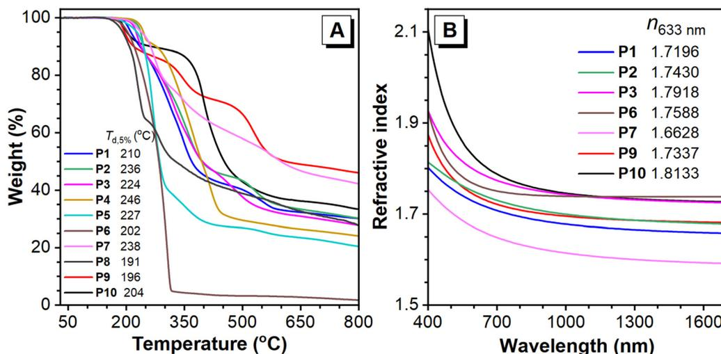
Fig. 7 (A) TGA thermograms of **P1**–**P10**, upon heating from  $50\text{ }^\circ\text{C}$  to  $800\text{ }^\circ\text{C}$  with a heating rate of  $10\text{ }^\circ\text{C min}^{-1}$  under  $\text{N}_2$ , and (B) the wavelength-dependent refractive indices of thin films from  $400\text{--}1700\text{ nm}$ .
