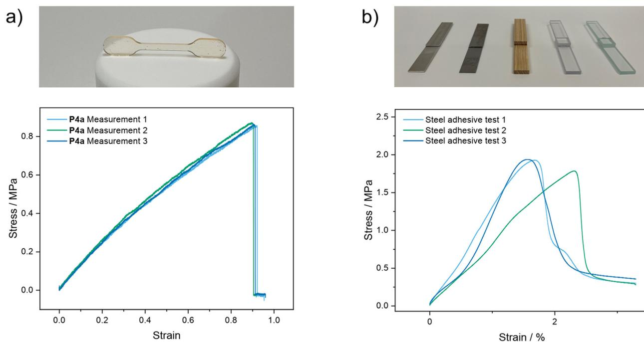
**Fig. 4** Dog bone sample of polymer **P4a** with the associated tensile strength measurements (a) and adhesive test samples prepared from polymer **P5a** and different substrates (aluminum, stainless, wood, PMMA, and borosilicate glass) with the adhesive tests of stainless-steel after 2 h of curing at room temperature (b).
