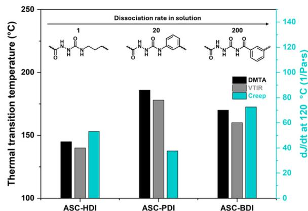
Fig. 8 Comparison of transition temperatures from DMTA and VTIR (left axis), the slope of  $J(t)$  at 120 °C (right axis) and model compound dissociation rate for ASC-HDI, ASC-PDI and ASC-BDI.
