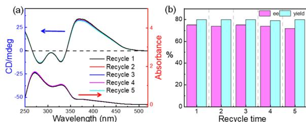
**Fig. 2** (a) The CD and UV-vis spectra of the recycled poly-**1**<sub>150</sub> measured in THF at 20 °C ( $c = 0.2 \text{ mg mL}^{-1}$ ). (b) Yield and ee values of the reaction between **4a** (0.20 mmol) and **5** (2.0 mmol) in toluene (0.5 mL) with  $(\text{CF}_3)_3\text{COH}$  (3.0 eq.) at  $-20^\circ\text{C}$  catalyzed by recycled poly-**1**<sub>150</sub> (with 20% loading).
