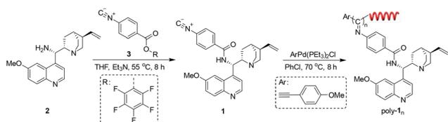
**Scheme 1** The route for the synthesis of the monomer 1 and poly-1<sub>*n*</sub>s.
