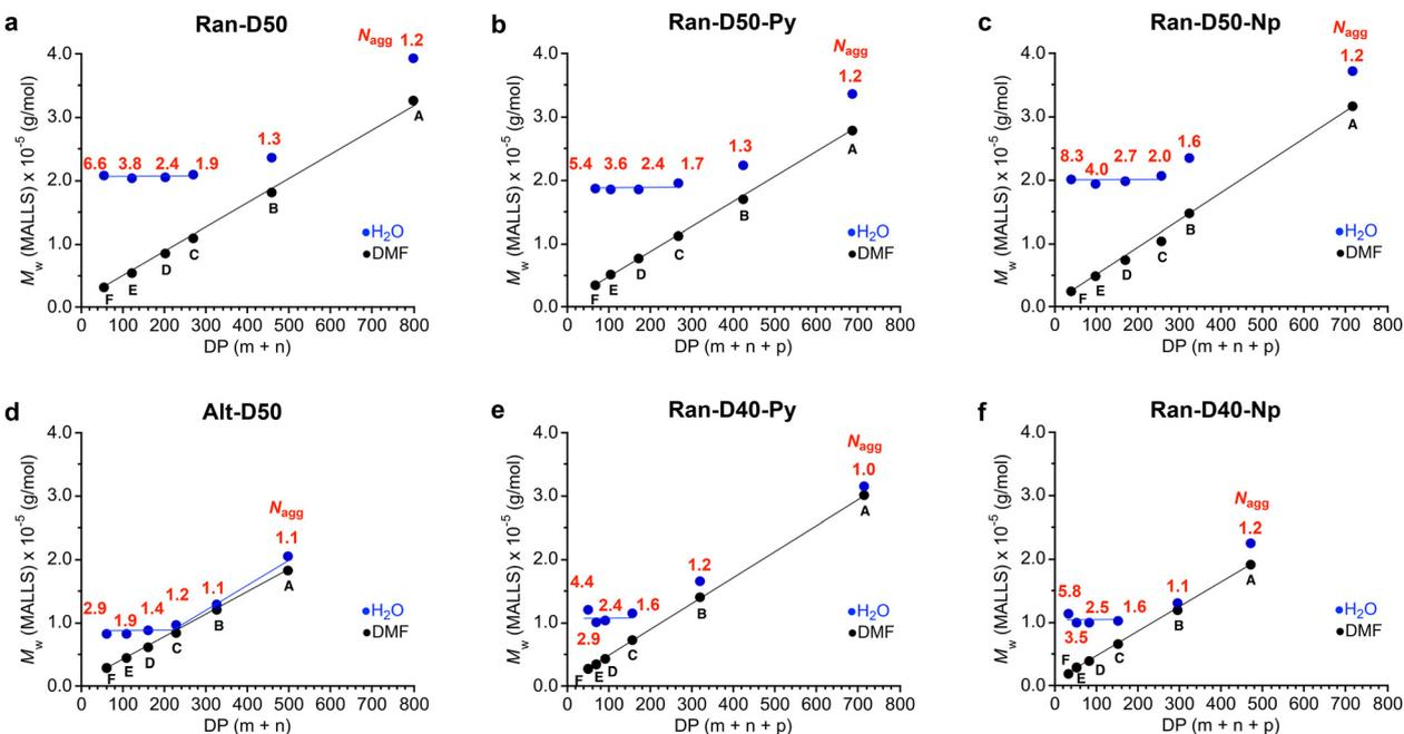
Fig. 4 Absolute weight-average molecular weight ( $M_w$ , determined by SEC-MALLS) of (a) **Ran-D50-A-F**, (b) **Ran-D50-Py-A-F**, (c) **Ran-D50-Np-A-F**, (d) **Alt-D50-A-F**, (e) **Ran-D40-Py-A-F**, and (f) **Ran-D40-Np-A-F** in water (100 mM NaCl, blue) or DMF (10 mM LiBr, black) as a function of the DP. Aggregation number:  $N_{agg} = M_{w,H_2O}/M_{w,DMF}$ .
