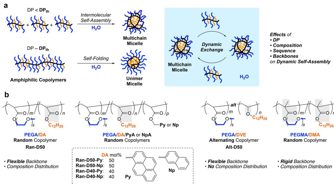
**Fig. 1** (a) Precision self-assembly of amphiphilic copolymers into multichain or unimer micelles in water, depending on the degree of polymerization (DP), and dynamic exchange of polymer chains between micelles. (b) Design of acrylate random, acrylate/vinyl ether alternating, and methacrylate random copolymers with hydrophilic poly(ethylene)glycol (PEG) chains and hydrophobic dodecyl groups.
