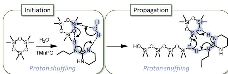
Scheme 1 “Proton shuffling” mechanism of initiation and propagation of  $D_3$  *via* TMnPG-catalyzed AROP.<sup>16</sup>
