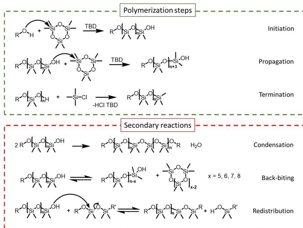
**Scheme 2** Polymerization steps and side reactions occurring during ring-opening polymerization (ROP) of hexamethylcyclorosiloxane using different types of initiators and TBD as a catalyst.<sup>6,16</sup>
