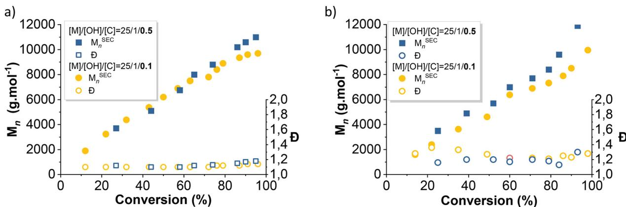
Fig. 7 Evolution of the number average molar mass and dispersity with  $D_3$  conversion of PDMS prepared by a TBD-catalyzed AROP of  $D_3$  initiated with (a)  $\Phi_2\text{Si}(\text{OH})_2$  and (b) Pdiol.
