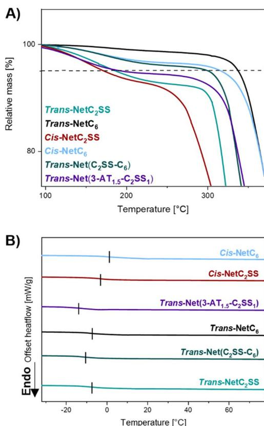
**Fig. 4** (A) TGA thermogram (25 °C – 600 °C, N<sub>2</sub>) of different networks synthesised in this work.  $T_{d,5\%}$  decreases with increasing disulfide bond content and higher *cis* content. (B) Zoomed in DSC thermograms (−30 °C to 80 °C, N<sub>2</sub>) of the second heating cycle of networks synthesised in this work.  $T_g$  highlighted by vertical dashes.
