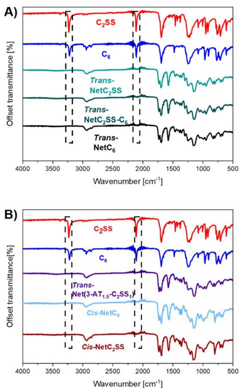
**Fig. 2** (A) FTIR spectra showing the disappearance of the alkyne stretching bands in the networks *trans*-NetC<sub>2</sub>SS, *trans*-Net(C<sub>2</sub>SS-C<sub>6</sub>), *trans*-NetC<sub>6</sub>. (B) FTIR spectra showing the disappearance of the alkyne stretching bands in the networks *trans*-Net(3-AT<sub>1.5</sub>-C<sub>2</sub>SS<sub>1</sub>), *cis*-NetC<sub>2</sub>SS, and *cis*-NetC<sub>6</sub>.
