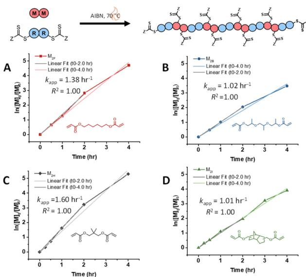
Fig. 3 Kinetic analysis of RAFT step-growth for diacrylate monomers with CTA<sub>2</sub>: (A) M<sub>2F</sub>, (B) M<sub>2G</sub>, (C) M<sub>2H</sub>, and (D) M<sub>2I</sub>.
