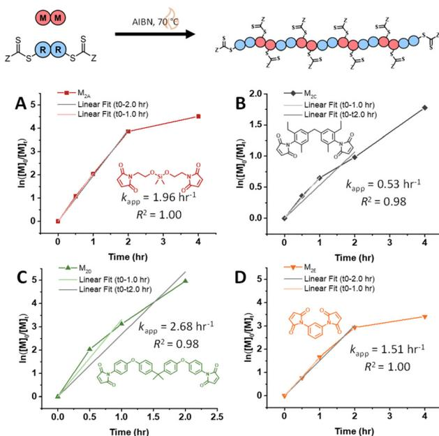
Fig. 2 Kinetic analysis of RAFT step-growth for maleimide monomers with CTA<sub>2</sub>: (A) M<sub>2A</sub>, (B) M<sub>2C</sub>, (C) M<sub>2D</sub>, and (D) M<sub>2E</sub>.
