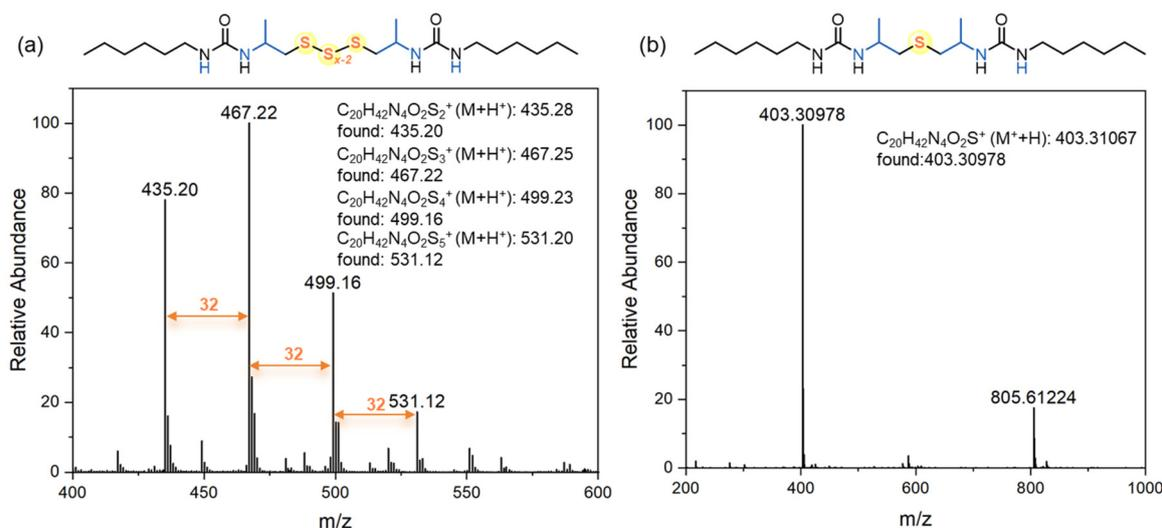
Fig. 2 (a) APCI MS spectrum of UA1-S<sub>x</sub>, and (b) HRMS spectrum of UA1-S.
