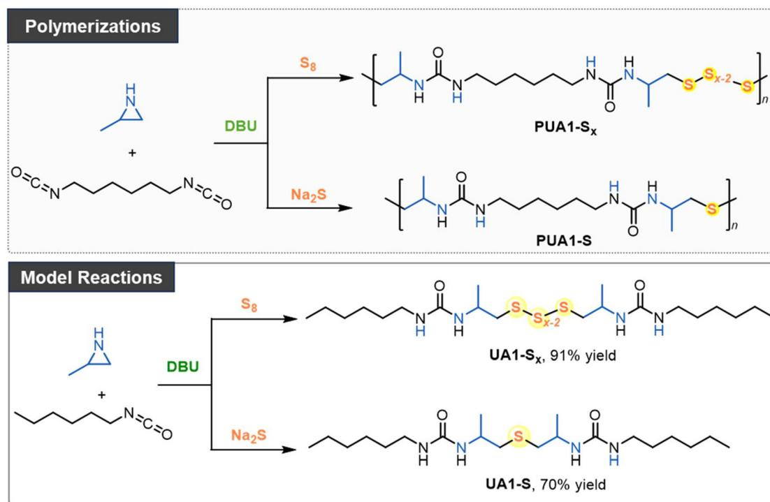
Scheme 1 Polymerizations and model reactions of aziridine, isocyanate, and inorganic sulfur.
