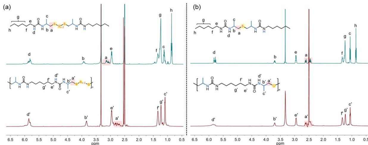
Fig. 1 <sup>1</sup>H NMR spectra of (a) UA1-S<sub>x</sub> and PUA1-S<sub>x</sub>, and (b) UA1-S and PUA1-S.
