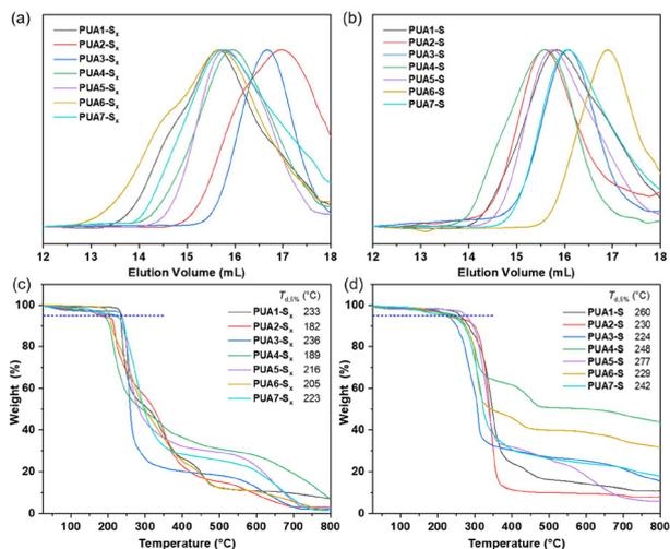
**Fig. 3** SEC traces of (a) PUA-S<sub>x</sub>, and (b) PUA-S. TG curves of (c) PUA-S<sub>x</sub>, and (d) PUA-S.
