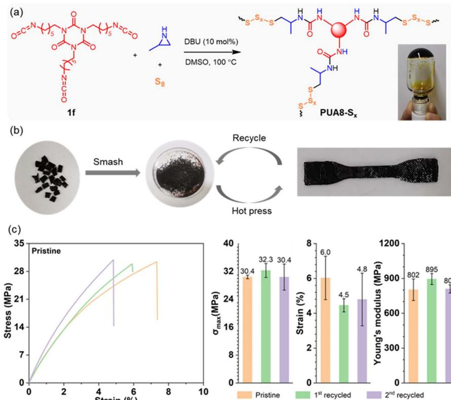
**Fig. 4** (a) Synthesis of polyurea vitrimer PUA8-S<sub>x</sub>. (b) The recycling process for the polyurea vitrimer sheet. (c) Stress–strain curves, maximum stress, breaking strain, and Young's modulus of vitrimer PUA8-S<sub>x</sub> before recycling and after two recycling cycles.
