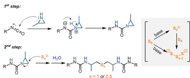
Scheme 2 A proposed mechanism for the cascade reaction.
