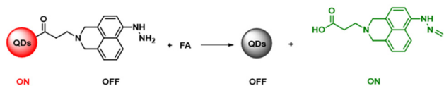
Scheme 5 Fluorescence quenching of QD-HBQP and fluorescence appearance of HBPQ after FA addition.
