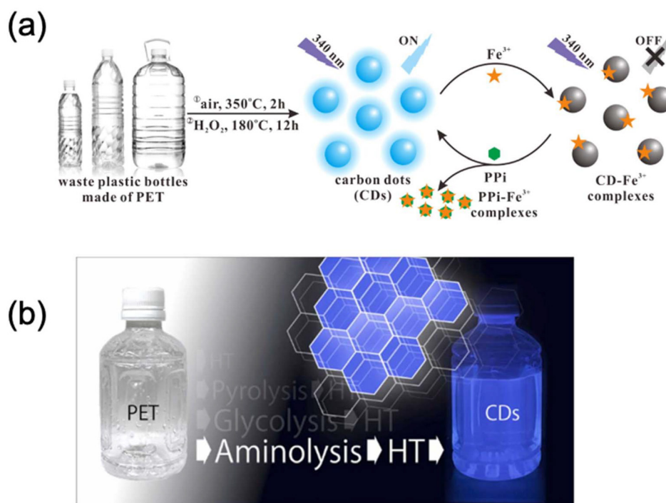
Fig. 6 (a) Schematic showing the green and low-cost synthesis of fluorescent CDs by a two-step process of air oxidation and hydrothermal reaction from waste PET and their use for “on–off–on” sensing of ferric and pyrophosphate ions by an electron transfer mechanism. Reprinted with permission from ref. 60. Copyright 2019 Elsevier. (b) Schematic of fluorescent PET-derived CDs with different preprocess approaches. Reprinted with permission from ref. 58. Copyright 2022 Elsevier.
