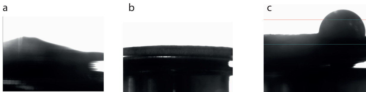
Fig. 6 Contact angle images of a water droplet placed on a pristine metallic lithium surface (a) and the P(S- r -MMA) copolymer brush-coated lithium surface (c), demonstrating its improved stability. For reference, the P(S- r -MMA) copolymer coated lithium surface is shown without a water droplet (b).
