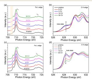
Fig. 2 NEXAFS spectra of LaFeO<sub>3</sub> and La<sub>0.67</sub>Sr<sub>0.33</sub>FeO<sub>3</sub> with different CV cycles. (a) Fe L-edge of LaFeO<sub>3</sub>, (b) O K-edge of LaFeO<sub>3</sub>, (c) Fe L-edge of  $La_{0.67}Sr_{0.33}FeO_3$  and (d) O K-edge of  $La_{0.67}Sr_{0.33}FeO_3$ . The yellow bars in (a) indicate the changes in the characteristics of Fe<sup>3+</sup> and Fe<sup>4+</sup> at 708 eV under different CV cycles.
