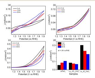
Fig. 5 OER performance of La<sub>1-x</sub>Sr<sub>x</sub>FeO<sub>3</sub> with different CV cycles. (a) CV polarization curves of LaFeO<sub>3</sub>, (b) CV polarization curves of La<sub>0.67</sub>Sr<sub>0.33</sub>FeO<sub>3</sub>, (c) CV polarization curves of La<sub>0.2</sub>Sr<sub>0.8</sub>FeO<sub>3</sub> and (d) current density of  $La_{1-x}Sr_xFeO_3$  (x = 0, 0.33, 0.8) with different CV cycles at +1.8 V (vs. RHE).
