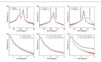
Fig. 1 XRD and XRR of La<sub>1-x</sub>Sr<sub>x</sub>FeO<sub>3</sub> thin films in pristine state (black curves) and after 30 CV cycles (red curves). (a) XRD of LaFeO<sub>3</sub>, (b) XRD of  $La_{0.67}Sr_{0.33}FeO_3$ , (c) XRD of  $La_{0.2}Sr_{0.8}FeO_3$ , (d) XRR of  $LaFeO_3$ , (e) XRR of  $La_{0.67}Sr_{0.33}FeO_3$  and (f) XRR of  $La_{0.2}Sr_{0.8}FeO_3$ .
