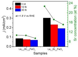
Fig. 6 Relationship between current density and Sr concentration of La<sub>0.67</sub>Sr<sub>0.33</sub>FeO<sub>3</sub> and La<sub>0.2</sub>Sr<sub>0.8</sub>FeO<sub>3</sub> with different CV cycles.
