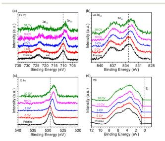
Fig. 3 SXPS of LaFeO<sub>3</sub> with kinetic energy constant at 550 eV. (a) Fe 2p, (b) La 3d, (c) O 1s and (d) VB spectra after different CV cycles.
