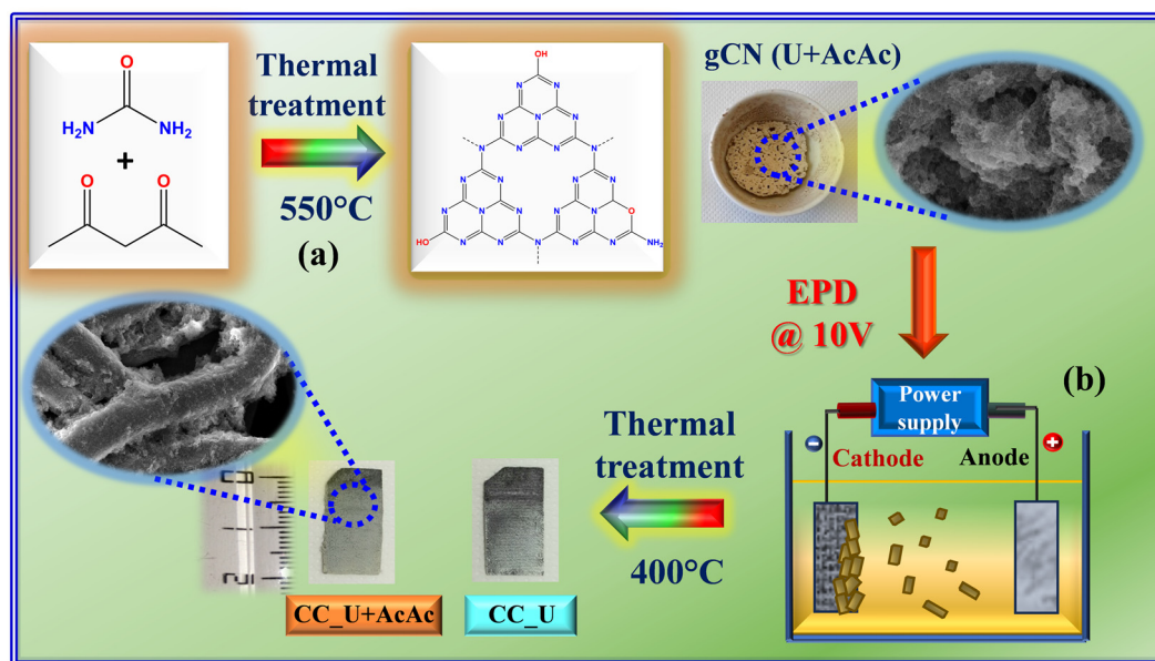
Scheme 1 Sketch of the procedure adopted in the present work for (a) the synthesis of gCN powders and (b) the subsequent preparation of gCN-containing electrode materials. U = urea; AcAc = acetylacetone; CC = carbon cloth; EPD = electrophoretic deposition. The suspensions for EPD were prepared by dispersing 40 mg of finely grinded carbon nitride powders into a beaker containing 50 mL of acetone and 4 mg of freshly dissolved I 2 (Sigma-Aldrich, ≥99.8%), followed by sonication for 30 min. For more details on the experimental procedures, see ESI,† §S1.
