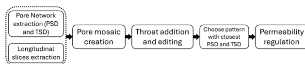
Fig. 1 Proposed steps for rock pattern design method.
