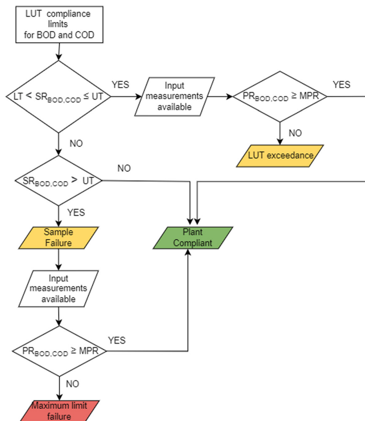
Fig. 2 Subset of the logic diagram for the compliance regulations on WRRFs.
