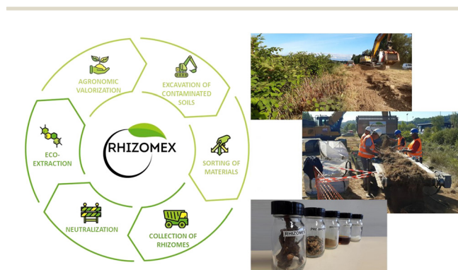
Fig. 4 Illustration of the circular economy approach by Rhizomex from the collection to the valorization of Japanese knotweed rhizomes. The diagram was kindly authorized for use by the Rhizomex company. Pictures were taken by the author.
