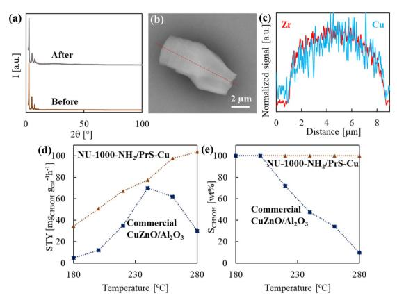
Fig. 7 Characterization and results of the sample tested for thermocatalysis: (a) PXRD of NU-1000-NH<sub>2</sub>/PrS-Cu before and after testing, (b and c) SEM image and Zr vs. Cu EDS line scan of NU-1000-NH<sub>2</sub>/PrS-Cu after testing, and (d) MeOH space-time yield (STY) and (e) MeOH selectivity  $(S_{CH-OH})$  of NU-1000-NH<sub>2</sub>/PrS-Cu compared to commercial CuZnO/Al<sub>2</sub>O<sub>3</sub> at the different studied temperatures.
