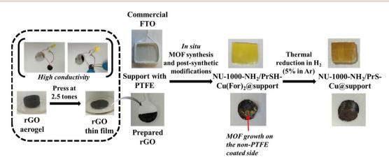
Fig. 2 Schematic representation of NU-1000-NH<sub>2</sub>/PrS-Cu@support preparation.
