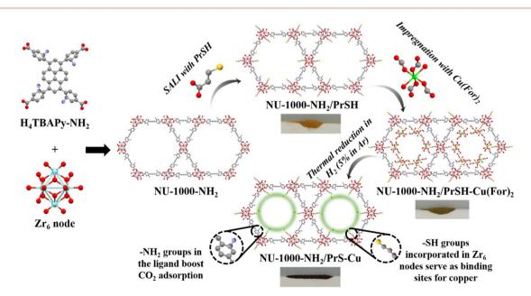
Fig. 1 Schematic representation of the followed steps to synthesize  $NU-1000-NH_2/PrSH-Cu$ , emphasizing in the purpose of the installed functionalities and including the color variation of the powder.
