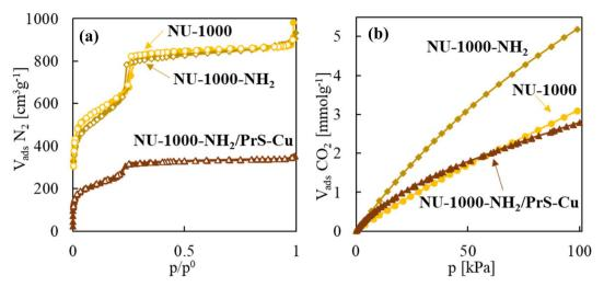
Fig. 3 Adsorption behavior: (a) N<sub>2</sub> adsorption-desorption isotherms at -196 °C and (b) CO<sub>2</sub> adsorption isotherms at 0 °C of the studied samples compared to pristine NU-1000.
