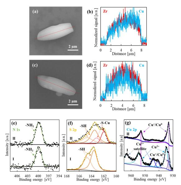
Fig. 4 Characterization before and after thermal reduction: SEM images and Zr vs. Cu EDS line scans of (a and b) NU-1000-NH $_2$ /PrSH-Cu(For) $_2$  and (c and d) NU-1000-NH $_2$ /PrS-Cu, respectively; and XPS spectra of (I) NU-1000-NH $_2$ /PrSH-Cu(For) $_2$  and (II) NU-1000-NH $_2$ /PrS-Cu in the (e) N $_{1s}$ , (f) S $_{2o}$  and (g) Cu $_{2o}$  regions, displaying the respective deconvoluted peaks.
