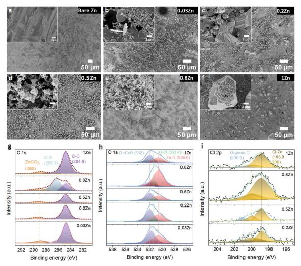
Fig. 5 Morphology evolution and surface composition of Zn electrodes after 20 cycles of Zn plating/stripping in different WISEs at 1 mA cm $^{-2}$  and 0.5 mA h cm $^{-2}$ . SEM images of (a) bare Zn and a cycled Zn anode in (b) 0.03, (c) 0.2, (d) 0.5, (e) 0.8, and (f) 1Zn electrolytes. The corresponding (g) C 1s, (h) O 1s, and (i) Cl 2p XPS spectra.
