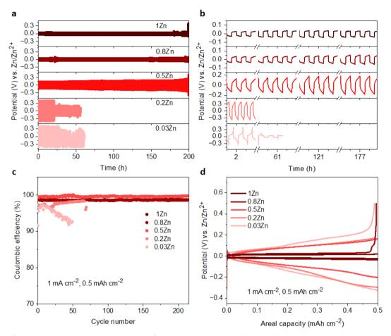
Fig. 4 Zn plating/stripping stability. Potential profiles for Zn $\|$ Zn cells obtained in 0.3, 0.2, 0.5, 0.8, and 1Zn electrolytes at current densities of (a) 2 mA cm $^{-2}$  and 0.5 mA h cm $^{-2}$  and (b) the corresponding overpotentials in different cycles. (c) CE of Zn plating/stripping on a Cu substrate in different electrolytes at 1 mA cm $^{-2}$  and 0.5 mA h cm $^{-2}$  current and capacity densities, respectively. (d) The corresponding potential profiles at the 40th cycle.
