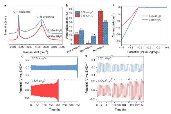
Fig. 6 Solvation structure and electrochemical stability of the Zn anode in 0.5Zn·4H<sub>2</sub>O electrolyte compared to concentrated 0.5Zn·2H<sub>2</sub>O. (a) Raman spectra in the water region. (b) The corresponding water population percentages. (c) LSV curves on a Ti substrate (d) Zn plating/stripping at 2 mA cm<sup>-2</sup> and 0.5 mA h cm<sup>-2</sup> in Zn||Zn symmetric cells and (e) the corresponding potential profiles.
