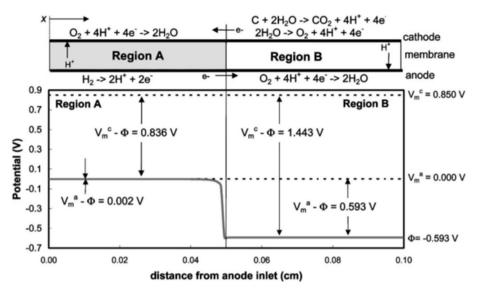
Fig. 1 Potential distributions along the anode flow path under reverse current conditions, where  $V_{\rm m}^{\rm c}$ ,  $V_{\rm m}^{\rm a}$  and  $\Phi$  denote the potential of cathode metal, anode metal and electrolyte, respectively. Reproduced with permission. Copyright 2005, The Electrochemical Society.
