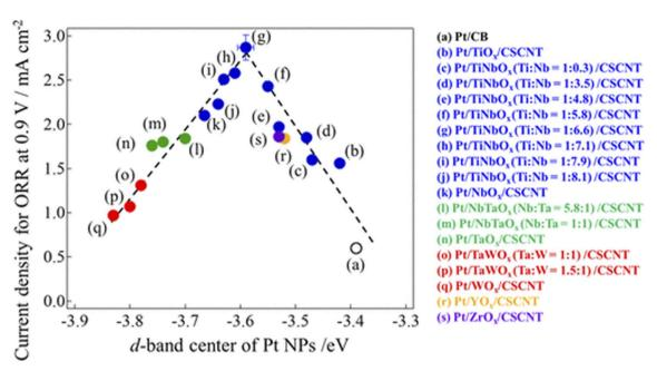
Fig. 7 Current density for the oxygen reduction reaction (ORR) at 0.9 V versus the d-band center of Pt nanoparticle curve. Reproduced with permission. Laboratory Copyright 2021, American Chemical Society.
