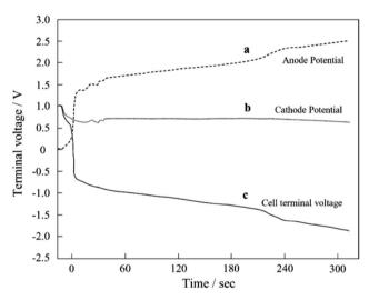
Fig. 2 (a) Anode potential, (b) cathode potential, and (c) cell voltage versus time curves during cell reversal. Reproduced with permission. Copyright 2004, Elsevier.
