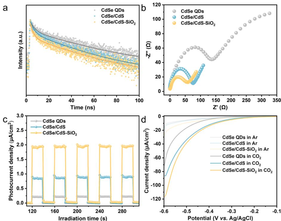
Fig. 4 (a) TRPL decay plots, (b) EIS plots and (c) transient photocurrent spectra of CdSe QDs, CdSe/CdS QDs and CdSe/CdS-SiO<sub>2</sub> composites. (d) LSV curves of CdSe QDs, CdSe/CdS QDs and CdSe/CdS-SiO<sub>2</sub> composites under Ar or CO<sub>2</sub> atmospheres.
