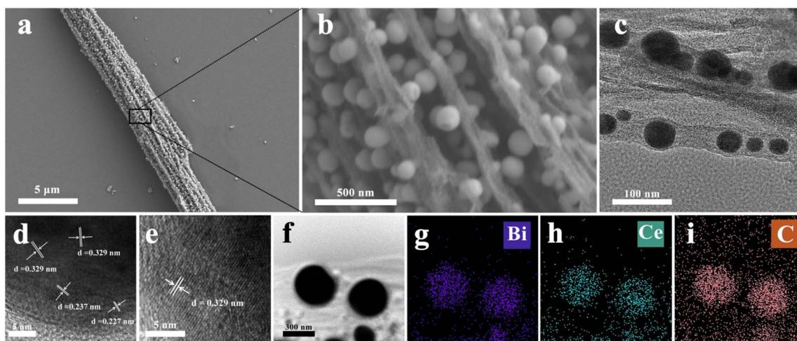
Fig. 1 Microstructure characterization of Ce<sub>2</sub>-Bi@C. (a) SEM image. (b) Localized magnified image of (a). (c) TEM image. (d and e) HRTEM images. (f-i) EDS mappings.
