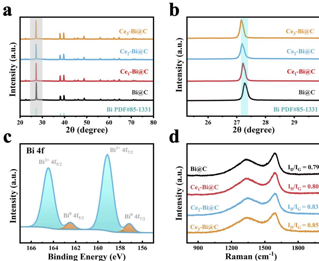
Fig. 2 (a) XRD patterns and (b) enlarged XRD patterns of Bi@C, Ce<sub>1</sub>-Bi@C, Ce<sub>2</sub>-Bi@C and Ce<sub>3</sub>-Bi@C. (c) Bi 4f XPS spectra of Ce<sub>2</sub>-Bi@C. (d) Raman spectra of various Bi-based composites.
