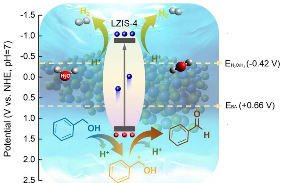
Fig. 7 A schematic of LZIS-4 in the dual coupling reaction of H<sub>2</sub> evolution and benzyl alcohol oxidation.
