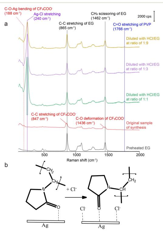
Fig. 5 (a) Raman spectrum of preheated EG and SERS spectra recorded from the original reaction solution of Ag irregular particles synthesized using  $CF_3COOAg$  and after it had been diluted with HCl/EG at various ratios, with the final concentration of  $Cl^-$  being 0.21 mM; and (b) schematic showing the effect of chemisorbed  $Cl^-$  on the orientation of C=O group of PVP relative to the Ag surface.
