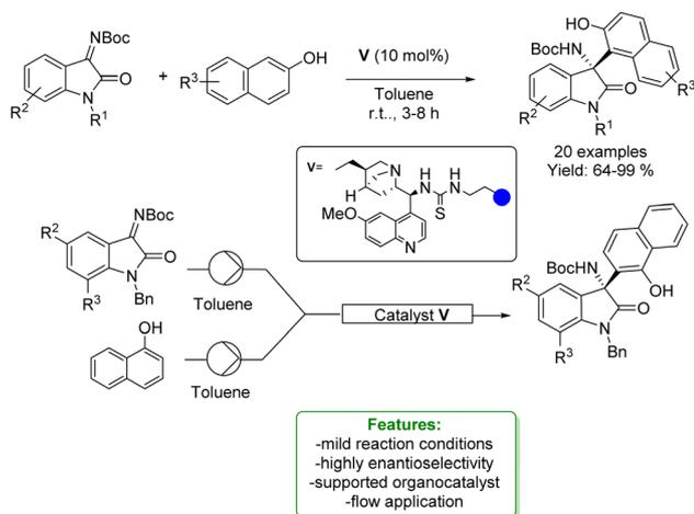
Scheme 44 Supported bifunctional chiral thiourea-based catalyst catalysed aza-Friedel–Crafts addition of naphthols with isatin-derived ketimines.<sup>132</sup>
