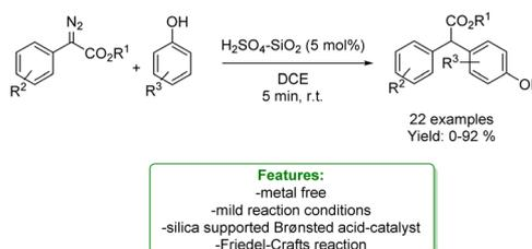
Scheme 16 Friedel-Crafts reaction of phenols catalysed by a supported Brønsted acid.<sup>77</sup>
