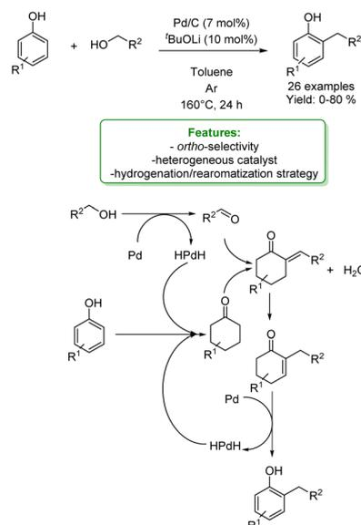
Scheme 1 Pd-catalysed alkylation of phenols with alcohols.<sup>54</sup>
