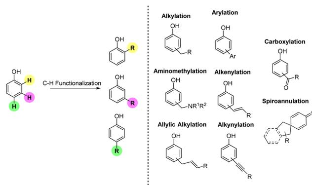
Fig. 2 The potential of Csp<sup>2</sup>-H functionalization of phenols.
