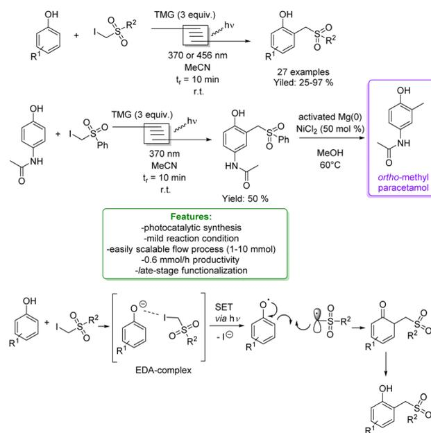
**Scheme 29** Alkylation of phenol with  $\alpha$ -iodosulfones *via* a photocatalytic flow strategy.<sup>102</sup>
