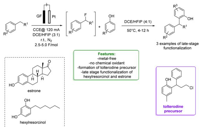
Scheme 31 Sequential electrochemical Csp<sup>3</sup>-H fluorination followed by metal-free benzylation of phenols.<sup>104</sup>
