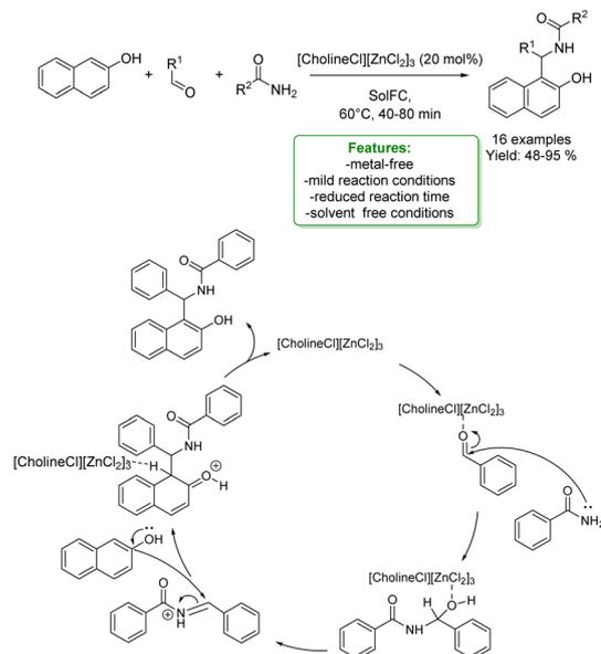
Scheme 40 Deep eutectic solvent catalysed three-component synthesis of 1-amidoalkyl naphthols.<sup>127</sup>
