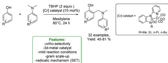
Scheme 32 Cr-catalysed *ortho*-aminomethylation of phenols with *N,N*-dimethylaniline.<sup>116</sup>
