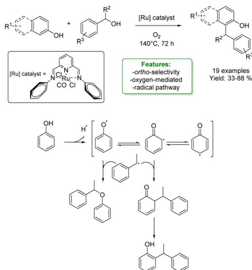
Scheme 3 Ru-catalysed alkylation of phenols with benzylic alcohols.<sup>56</sup>
