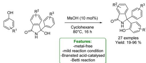
Scheme 45 Brønsted acid-catalyzed Betti reaction of phenols with isoindolinone alcohol.<sup>133</sup>
