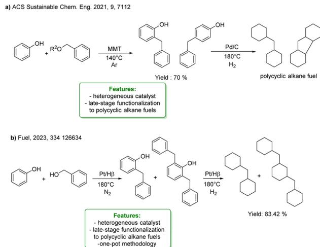
**Scheme 28** Acid-catalysed alkylation of phenol, and subsequent HDO to obtain bi- or poly-cycloalkanes or high-density biofuels (a) two-step synthesis of perhydrofluorene, from phenols and benzyl acetate catalysed by solid acid montmorillonite (MMT), and Pd/C.<sup>98</sup> (b) One-pot strategy for preparing polycyclic alkane from phenol and benzyl alcohol over a bifunctional Pt/H $\beta$  catalyst.<sup>99</sup>
