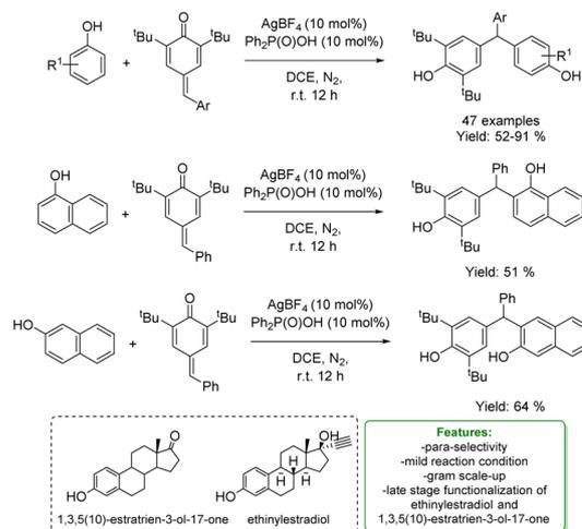
Scheme 13 Ag-catalysed *para*-selective 1,6-hydroarylation of *para*-quinone methides with phenols and naphthols.<sup>71</sup>
