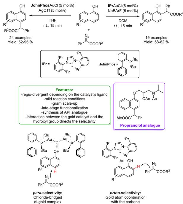
Scheme 6 Regio-divergent alkylation of phenols and naphthol with  $\alpha$ -aryl- $\alpha$ -diazoesters catalysed by a Au-catalyst.<sup>63</sup>
