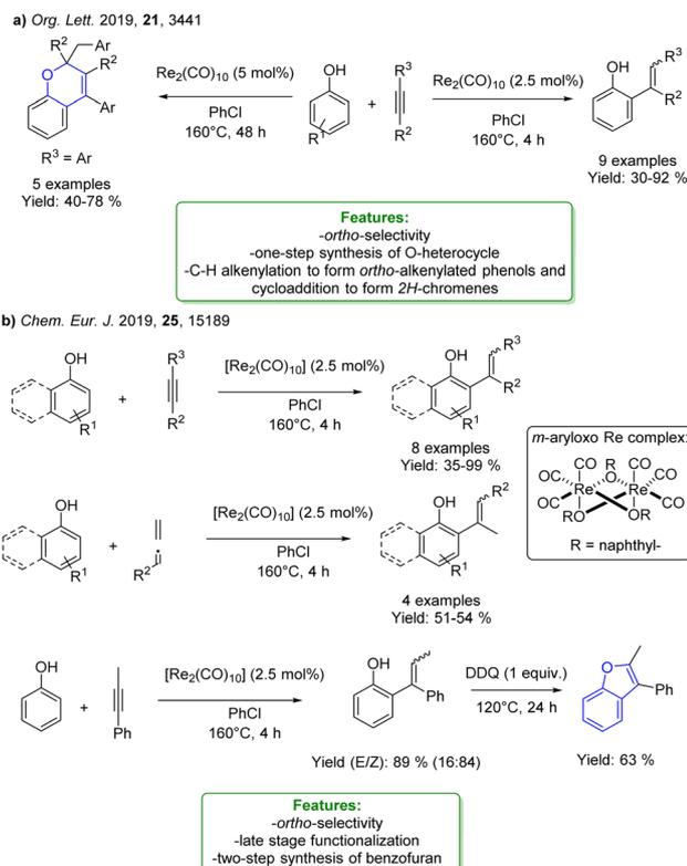
Scheme 62 Re-catalysed *ortho*-alkenylation of phenols with alkynes and cyclization to 2*H*-chromene.<sup>181,182</sup>
