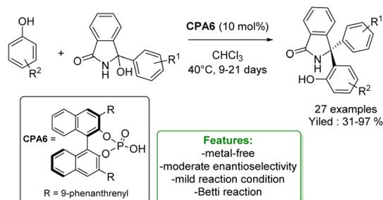
Scheme 46 Chiral phosphoric acid-catalyzed Betti reaction of phenols with isoindolinone alcohol.<sup>134</sup>
