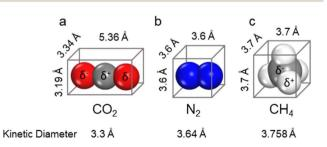
Scheme 4 Physical and chemical properties of CO<sub>2</sub> (a), N<sub>2</sub> (b), and  $CH_4$  (c).
