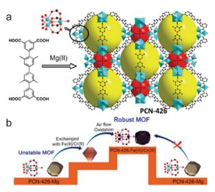
Fig. 17 (a) The ligand and the structure of PCN-426-Mg; (b) the metal exchange routes for PCN-426. Reproduced from ref. 161 with permission from the American Chemical Society, Copyright 2014.
