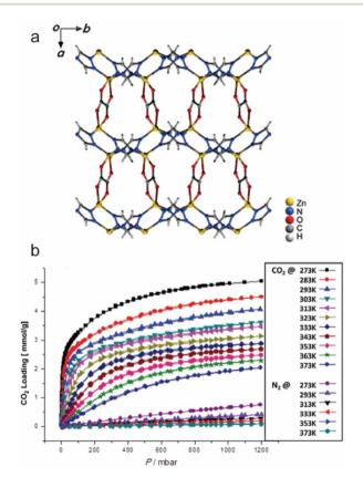
Fig. 35 (a) The structure of CALF-20. (b) The  $\rm CO_2$  and  $\rm N_2$  isotherms of CALF-20 at different temperatures. Reproduced from ref. 217 with permission from the Advancement of Science, Copyright 2021.
