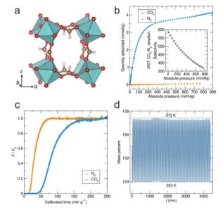
Fig. 31 The structure and CO<sub>2</sub> adsorption performance of ALF. Reproduced from ref. 210 with permission from the Advancement of Science, Copyright 2022. (a) The structure of ALF. (b) The CO<sub>2</sub>/N<sub>2</sub> sorption isotherms of ALF at 298 K. (c) The breakthrough curves of ALF at 323 K. (d) 130 cycles of adsorption and desorption.
