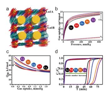
Fig. 32 (a) The structure of NKMOF-3-Ln. (b)–(d) The  $\rm CO_2/N_2$  adsorption isotherms,  $\rm CO_2$  adsorption enthalpy, and breakthrough curves of  $\rm CO_2/N_2$  (15/85) mixtures at 298 K. Reproduced from ref. 212 with permission from the American Chemical Society, Copyright 2019.
