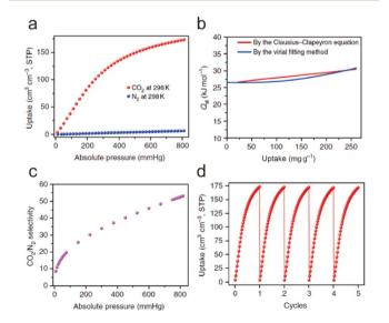
Fig. 34 (a) The  $CO_2$  and  $N_2$  adsorption isotherms for FJI-H14 at 298 K. (b) The isosteric heat of  $CO_2$  adsorption ( $Q_{st}$ ) for FJI-H14. (c) The IAST selectivity of FJI-H14 for  $CO_2/N_2$  (15:85). (d) 5 Cycles of  $CO_2$  adsorption for FJI-H14 at 298 K. Reproduced from ref. 136 with permission from Springer Nature, Copyright 2017.
