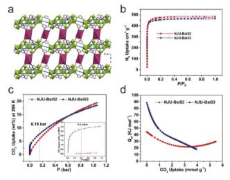
Fig. 37 (a) The structure of NJU-Bai52 and NJU-Bai53. (b) The  $N_2$ sorption isotherms of NJU-Bai53 (77 K) before and after water treatment. (c) The CO<sub>2</sub> adsorption isotherms of NJU-Bai52 and NJU-Bai53 at 298 K. (d) The adsorption enthalpy of NJU-Bai52 and NJU-Bai53 for CO<sub>2</sub>. Reproduced from ref. 233 with permission from the American Chemical Society, Copyright 2019.
