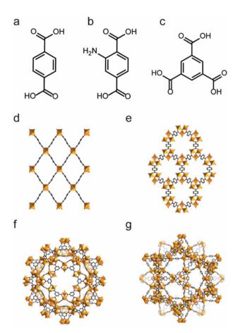
Fig. 1 The structures of the MIL series and the used ligands. (a) The  $H_2BDC$  ligand. (b) The  $H_2BDC$ -NH<sub>2</sub> ligand. (c) The 1,3,5-BTC ligand. (d) MIL-53. (e) MIL-88. (f) MIL-100. (g) MIL-101. Reproduced from ref. 144 with permission from Wiley, Copyright 2018.
