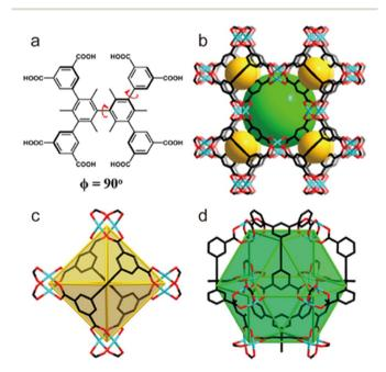
Fig. 19 (a) Structure of the ligand  $H_8$ tdhb, (b) crystal structure of BUT-155a, and (c) octahedral cage (cage A) and (d) cuboctahedral cage (cage B) in BUT-155a (color code: C, black; O, red; Cu, blue; H atoms on ligands are omitted for clarity). Reproduced from ref. 164 with permission from the American Chemical Society, copyright 2017.
