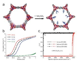
Fig. 40 (a) Introducing  $N_2H_4$  into pores of  $Mg_2(dobdc)$ . (b) The  $CO_2$  sorption isotherms of  $(Mg_2(dobdc)(N_2H_4)_{1.8})$  at different temperatures. (c) The breakthrough curves of  $(Mg_2(dobdc)(N_2H_4)_{1.8})$  for  $CO_2/N_2$  (1: 999) under different humid conditions. Reproduced from ref. 223 with permission from the Royal Society of Chemistry, Copyright 2016.
