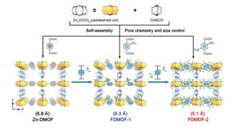
Fig. 20 Fluorinated functional group introduction into the confined pore space. Reproduced from ref. 166 with permission from Wiley, Copyright 2023.
