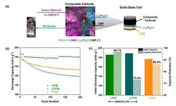
Fig. 5 (a) Fabrication of composite cathode and solid-state cell configuration, LTO/Li<sub>6</sub>PS<sub>5</sub>Cl/NMC-PE composite. (b) Specific discharge capacity vs. cycle number at T = 60 °C, 1 MPa stack pressure, 1 mA cm<sup>-2</sup>. (c) Initial discharge capacity, and capacity retention after 200 cycles (labelled).
