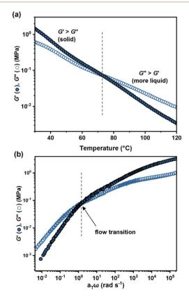
Fig. 4 Viscoelastic mechanical properties for ABA (50, 0.35)/LiTFSI. (a) Temperature-dependence of G' and G''. (b) Master curve of the frequency dependence of G' and G''.
