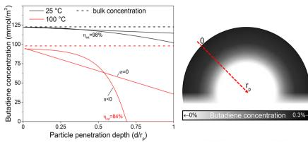
Fig. 6 Schematic intraparticle concentration gradient. Estimated butadiene concentration as function of penetration depth into an exemplary catalyst grain. Calculated by eqn (15) (n = 0) or eqn (16) (n < 0). Bulk concentration calculated from the ideal gas law at 1 atm. Surface concentration estimated from Carberry number for 180 µm grains (eqn (S23)†). The grayscale in the inset illustrates the radial concentration inside a spherical catalyst grain with  $\eta_{\rm int}$  = 84% (n < 0).
